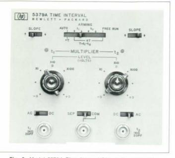
**Fig. 3.** Model 5379A Time-Interval Plug-in is used with the computing counter to measure time intervals with  $\pm 1$  ns accuracy and  $\pm 0.1$  ns resolution. Intervals down to zero can be measured, and if the stop pulse ( $t_1$  input) occurs before the start pulse ( $t_1$  input) the display will have a minus sign.
