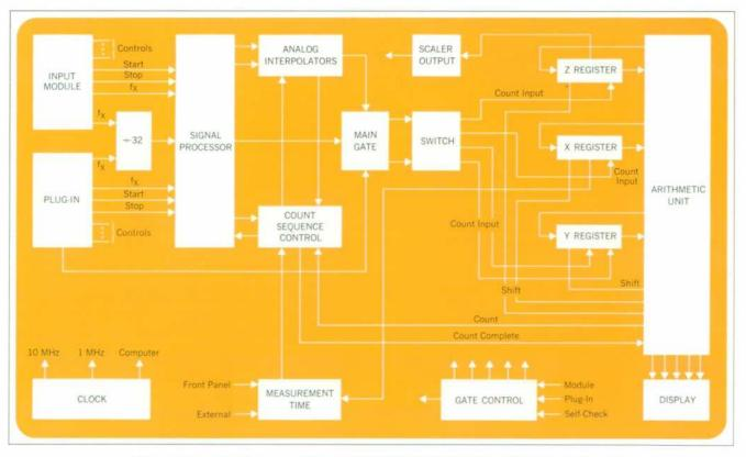
Fig. 1. Analog interpolators in the Model 5360A Computing Counter reduce the ±1 count uncertainty by a factor of 1000. The arithmetic unit provides the computational capability needed to make use of interpolation. When the counter is counting, the X, Y, and Z registers act as decade counting assemblies.
