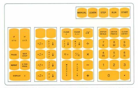
**Fig. 5.** This is the key configuration of the Model 10537A Keyboard which will be introduced later this year. With the computing counter, it gives the user anything from a desk calculator to a complete programmable measurement system capable of making multiple measurements and interprocessing them digitally before display. Applications include units conversion, computing phase and  $\Delta t/t$ , rms calculations, and many others.
