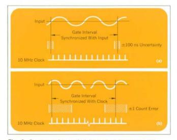
Fig. 2. By measuring period instead of frequency the automatic counter gets much better resolution at low frequencies than a direct-counting instrument with the same 10 MHz clock rate. (a) Time-interval (period) measurement of N input cycles. Resolution is a constant 100 ns for any input frequency. (b) Direct frequency count. Resolution is  $\pm 1$  count of the input frequency.
