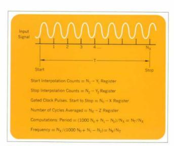
**Fig. 3.** For period and frequency measurements the computing counter's measurement cycle is synchronized with the input signal. The selected measurement time is actually a minimum value; the actual time is an integral number of input periods. Besides measuring  $T_{0r}$ ,  $T_{1r}$ , and  $T_{2}$  as for time interval, the counter counts the input periods  $N_{x}$  and then computes period or frequency.
