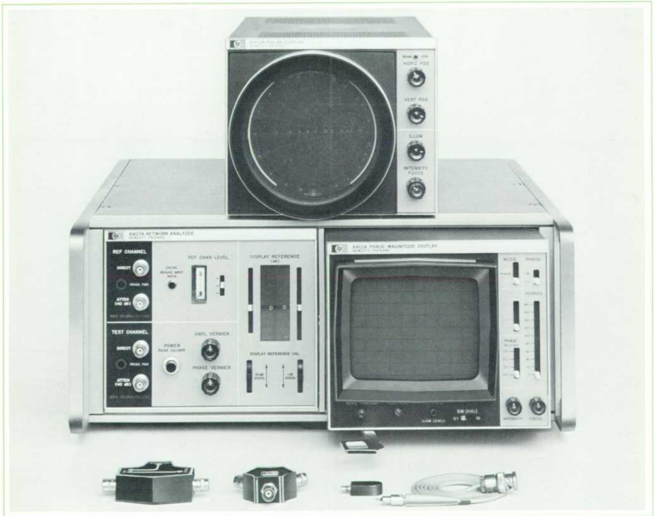
Fig. 1. Network analyzer system for range 0.1 to 110 MHz includes optional plug-in displays. Two are shown here, Model 8412A Phase-Magnitude (partly installed) and Model 8414A Polar (above). In the foreground (left) is a new directional bridge with more than 40 dB directivity across the band of concern. Also shown are power splitter, passive probe and divider, parts of the transducer kits designed for the system.
