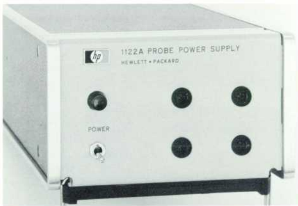
Fig. 5. Model 1122A Probe Power Supply, for use where instruments are not equipped to power Probe, furnishes power for up to four Model 1120A Probes.
