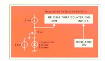
Fig. 10. Units conversion with Model 5326B. The temperature of the diode can be read directly in °C with 0.1°C resolution. The channel A input normalizes the reading.
