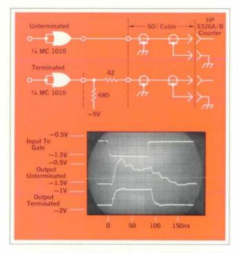
Fig. 3. Output of an ECL gate connected to Model 5326A Timer/Counter, first using only a 50 $\Omega$  cable (middle trace) and then a 50 $\Omega$  cable with the proper series termination. Reflections resulting from improper termination can cause double counts, incorrect readings.
