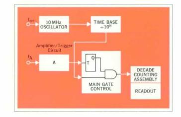
Fig. 5. Period and period-ratio measurements are the inverse of frequency and frequency-ratio measurements.
