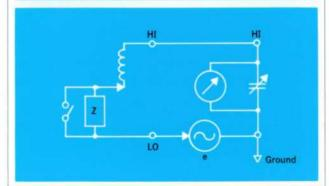
Fig. 7. Three ways in which components are measured with the Q meter. Most components in the medium inductance range (0.09  $\mu$ H to 1.2 H) are connected directly (a). High impedance components are connected in parallel (b) with the capacitor, and low impedance components use the series connection (c).
