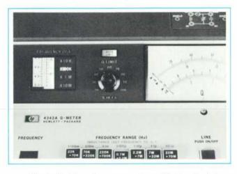
Fig. 8. Limit is set as a percentage of full scale. A lamp indicates Q over the limit.
