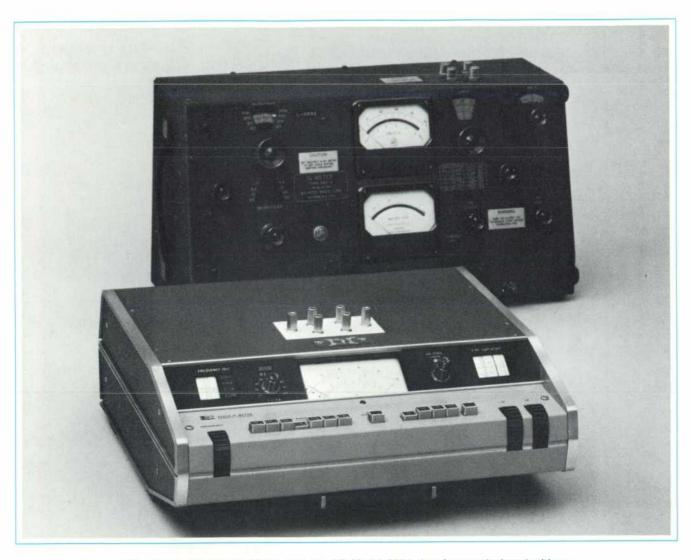
The classic Boonton Q Meter, now the HP Model 260A, has been redesigned with an extended Q range and circuit improvements that make it faster and easier to use.
