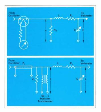
Fig. 4. Constant current injection system (a) used in the older Model 260A Q meter uses a thermocouple that can be easily damaged. Constant voltage injection system (b) used in the new Model 4342A Q Meter uses a transformer with an output impedance of only 1 milliohm.
