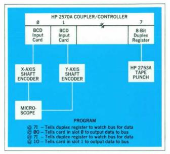
Fig. 5. The coupler / controller can also operate independently of any computing machine. In such applications it is programmed by its internal diode pinboard, by punched tape, or from a teleprinter keyboard. Here it is used to record the positions of objects on a microscope slide.
