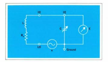
Fig. 1. A series resonant circuit is the basis of Q measurement.
