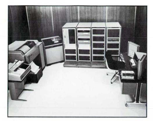
Fig. 1. HP 3000 Computer System has multilingual and multiprogramming capabilities usually found on much larger systems.
