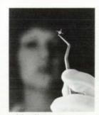
**Cover:** The tweezers hold a new monolithic silicon-onglass diode quad — four Schottky-barrier diodes arranged in a ring configuration (shown prior to encapsulation) for double-balanced mixer service. This construction achieves better matching and lower parasitics than has been possible
