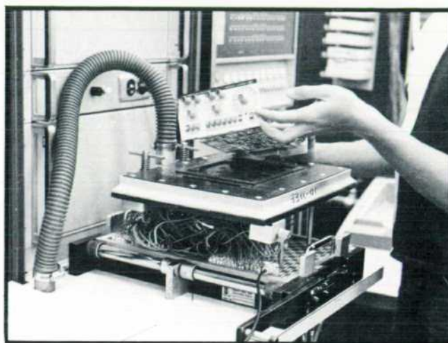
Fig. 4. Automatic test system quickly finds any production errors, reducing trouble-shooting time significantly. A vacuum holds the instrument on the test fixture and protruding component leads make contact through holes in the fixture.
