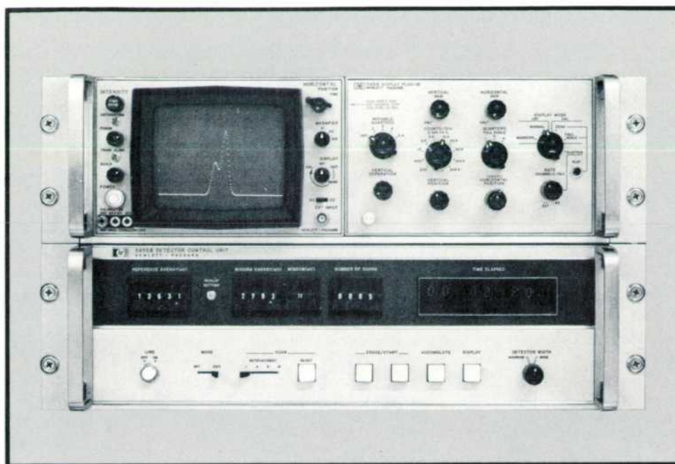
Fig. 10. Range of energies to be scanned, the starting energy, the scan rate, and the number of scans are selected at the detector control unit. The multichannel analyzer displays the resulting spectrum. Data can also be plotted or transmitted to a computer for analysis.
