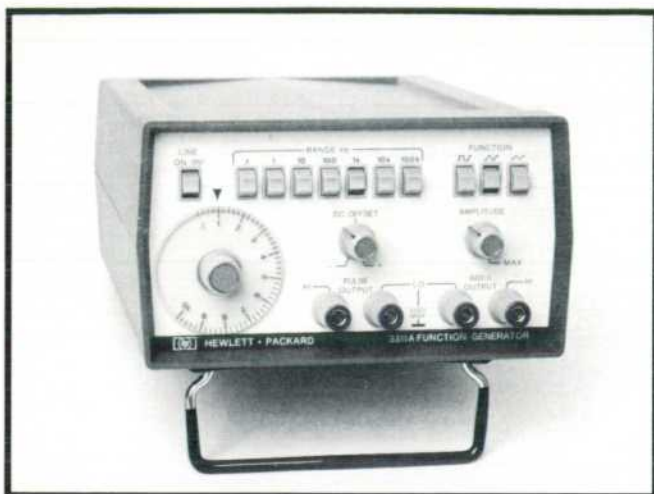
Fig. 2. New Model 3311A Function Generator supplies waveforms for many kinds of tests over 0.1 Hz to 1 MHz frequency range. Maximum output is 10V peak to peak into a 600 \Omega load (20V into an open circuit). The amplitude control has a range of 30 dB.
