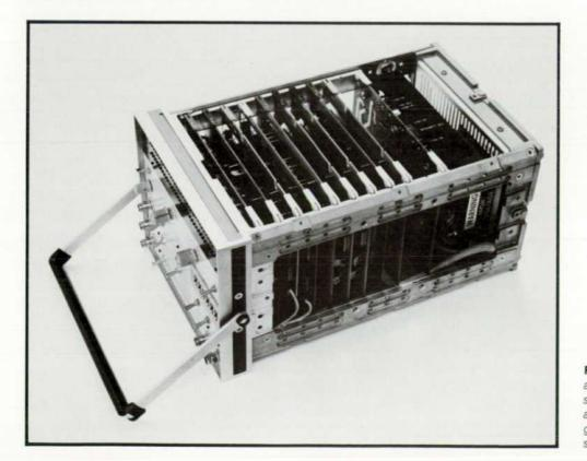
Fig. 13. Logic Analyzer is mechanically designed for ease of assembly and repair. Top, bottom, and sides are easily removed to gain access to all sides of the instrument.
