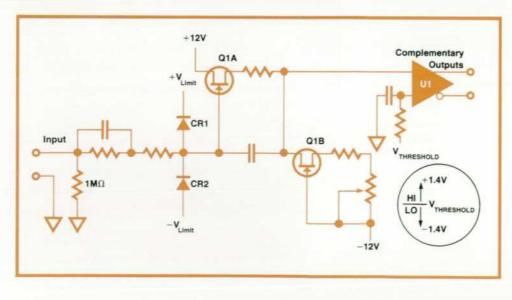
Fig. 7. High-impedance input amplifiers minimize circuit loading. Variable threshold assures compatibility with all IC logic families.
