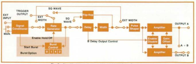
Fig. 5. Simplified block diagram of Model 8015A Pulse Generator.
