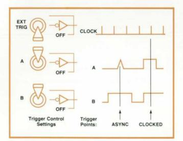
Fig. 10. In CLOCKED mode, the Logic Analyzer monitors its inputs for the trigger condition only at the selected clock edge. In ASYNC mode, triggering occurs as soon as the trigger condition appears at the inputs. Triggering is always edge-sensitive.
