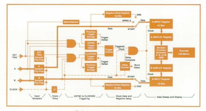
Fig. 9. Logic Analyzer block diagram.
