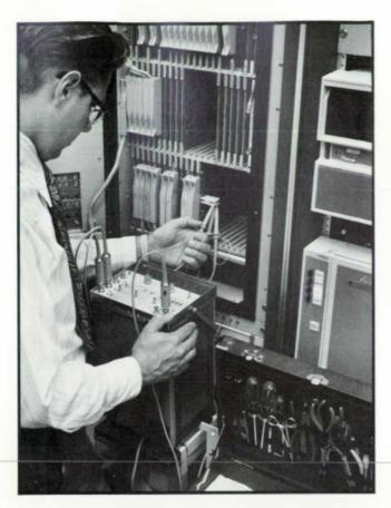
Fig. 14. Light weight, handle, and form factor make the Logic Analyzer suitable for field service applications.
