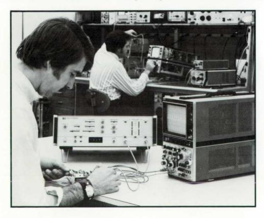
Fig.1. New Model 8015A 50 MHz Pulse Generator has two outputs with individual control of amplitude, polarity, and baseline level for each. The arrangement of the controls simplifies operation. The instrument shown here is equipped with the optional burst mode of operation. output current, especially useful when the generator is used to drive magnetic devices. The doubled current capability enables pulse swings of up to 30 V anywhere within a  $\pm 16$  V to  $\pm 16$  V window.
