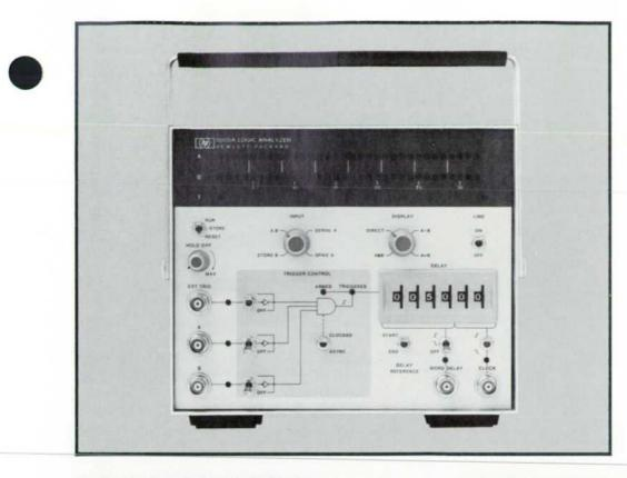
Fig. 1. Model 5000A Logic Analyzer's two rows of 32 light-emitting diodes display the sequences of logic states at the A and B inputs. Positive and negative delay, combinatorial triggering, storage, spike detection, and several display modes help solve a multitude of digital measurement problems in design and troubleshooting.
