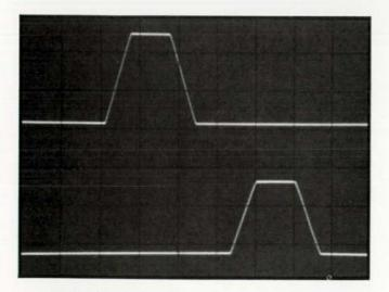
Fig. 2. Dual-trace oscillogram shows how pulses in channel B can be delayed with respect to channel A, giving two-phase clock pulses.
