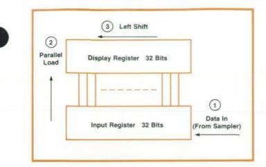
Fig. 11. Logic Analyzer displays data with oldest information at the left. At clock rates below 1 kHz the three steps shown occur on each clock cycle. The result is that each bit is displayed, properly positioned, as soon as it is entered. Data does not appear to shift in and is viewable while the display is being loaded.
