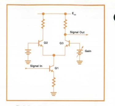
**Fig. 7.** Electronic attenuator splits the signal current into two paths. The proportion that goes to Q3 depends on Q3 bias. Q2 sinks the remainder.
