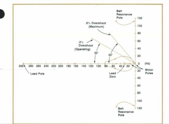
Fig. 4. Root-locus plot of the penpositioning servo system shows that the operating loop gain results in poles that have less than maximum overshoot but are still off the real axis. This results in the fastest possible response consistent with adequate gain margin for the belt resonance poles.
