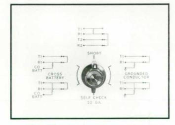
Fig. 4. 4913A fault mode switch is set to the type of fault.
