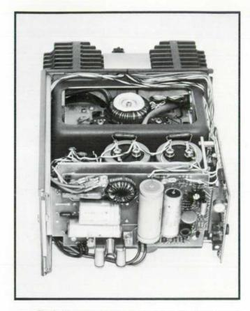
Fig. 2. Aluminum shield, cut open in this view, houses power transformer, switching transistors, and other sources of electrical interference.
