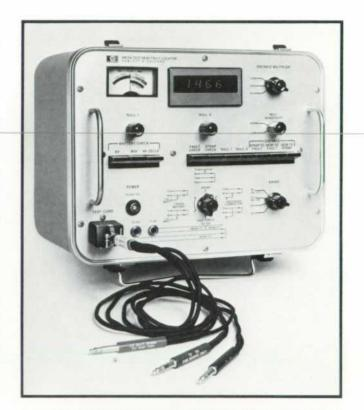
Fig. 1. Model 4913A Test Desk Fault Locator quickly locates shorts, crosses, and grounds without requiring special training. Piano-key switches are used in left-to-right sequence.
