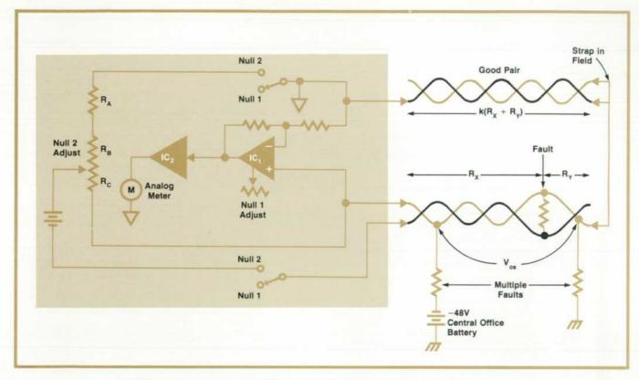
Fig. 5. Two nulls are adjusted in 4913A operation. Null 1 cancels voltages such as V<sub>os</sub> that often caused errors in the old three-Varley method. Null 2 sets up a balanced-bridge condition.
