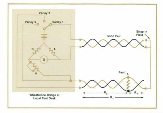
Fig. 3. Old three-Varley method required the test desk operator to make three Wheatstone-bridge nulls and calculate the distances represented by R<sub>X</sub>, R<sub>Y</sub>, and R<sub>T</sub>.
