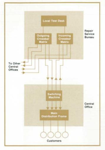
Fig. 2. 4913A Test Desk Fault Locator is designed for use at a local test desk in a telephone company repair service bureau. Faults are typically in customer lines originating in central offices. The test desk operator works with a craftsman in the field, e.g., at the customer location.
