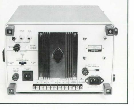
Fig. 8. Battery charger is connected across the internal batteries whenever the recorder is plugged into the ac line. When the rearpanel source switch is in the battery standby position, ac power can be used and the recorder will switch to battery power if the ac power fails.
