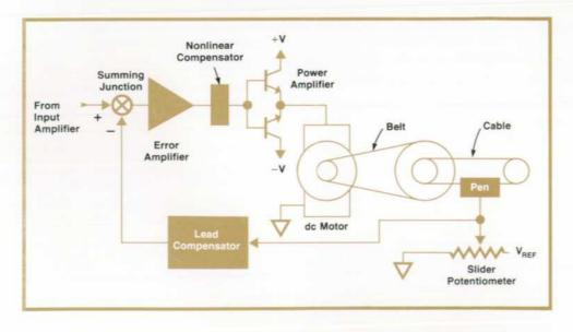
Fig. 3. Slider-potentiometer provides pen-position information for the servo system. Pens are disposable fiber-tip type, insensitive to attitude and acceleration, and the ink is specially formulated to write from −28°C to +65°C.
