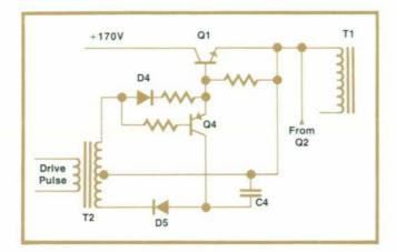
Fig. 6. The switching circuit speeds up turn-off of power transistor Q1.
