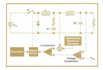
Fig. 4. By retaining the feedback loop around the first filter section, and adding a second loop around the second filter section, the new power supplies achieve relatively fast response with closely-regulated output.
