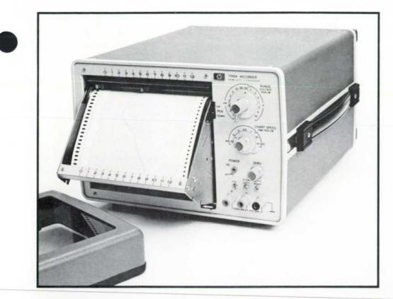
Fig. 1. Model 7155A Portable Strip-Chart Recorder is designed to deliver laboratory accuracy in field use. Pen displacement is accurate within  $\pm 0.5\%$  and chart speed is accurate within  $\pm 1\%$ , independent of ac line frequency, over a wide range of environmental conditions. Internal batteries are optional.
