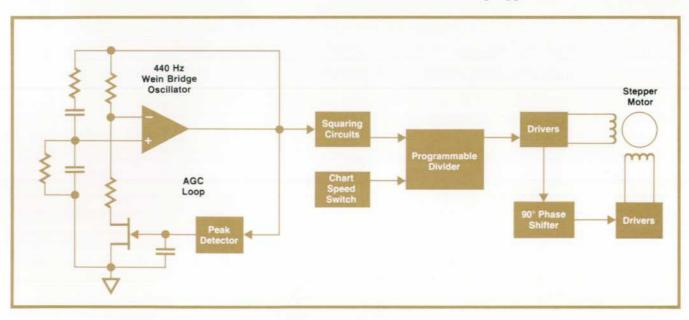
Fig. 6. Chart drive motor is a stepper motor driven by a Wien bridge oscillator with AGC. Seven chart speeds are derived by dividing the oscillator frequency. No mechanical transmission is needed. The oscillator makes chart speed independent of power line frequency and makes battery operation possible.
