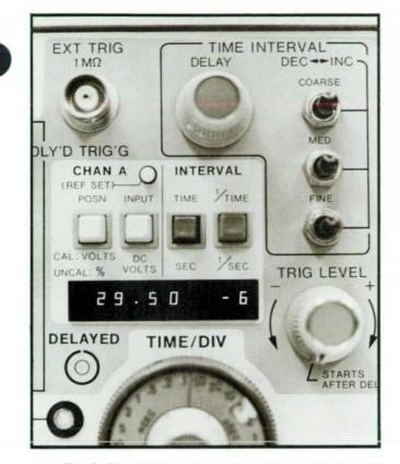
Fig. 5. The microprocessor is activated by pressing one of the function buttons (POSN, INPUT, TIME, 1/TIME). If any of the oscilloscope controls are not set appropriately for the measurement selected, the digital readout displays ".0".
