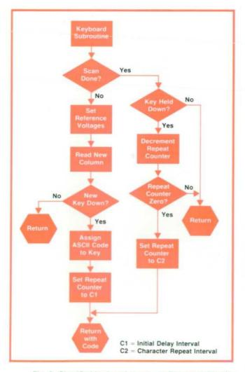
Fig. 3. Simplified keyboard scanner, a firmware subroutine called by the system monitor.
