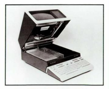
Fig. 1. Model 2640A Interactive Display Terminal operates in either character or page mode. Data transmission is compatible with EIA RS 232C and with Bell type 103 and 202 moderns. Data rates from 110 to 2400 baud are selectable. Character code for data transmission is ASCII.
