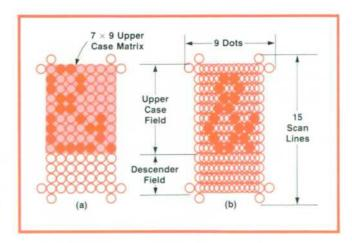
Fig. 1. Basic 2640A character cell is nine dots wide by fifteen scan lines high, including spaces between characters and rows. Diagram at left shows an alphanumeric character designed on the basic 7  $\times$  9 dot matrix. At right is the same character as it appears in the 2640A with the horizontal half-shift.
