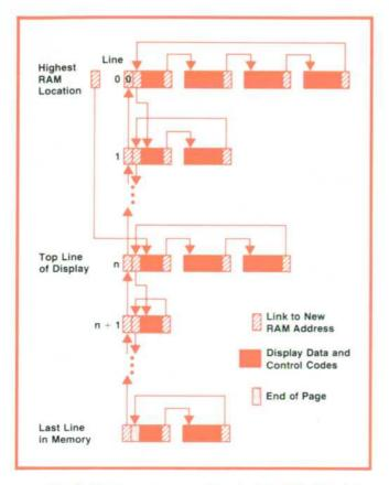
Fig. 2. Display memory consists of a linked list of fixed-size blocks of RAM. The display system starts at the first address on the screen and follows the list to produce an entire screen of information.
