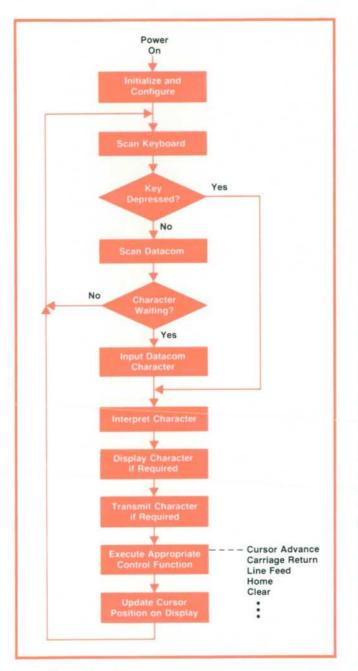
Fig. 1. The microprocessor normally executes a section of firmware called the system monitor, a basic loop in which the processor scans the keyboard and data communications interface and waits for something to happen. When a key is pressed or a character received, the appropriate subroutine is executed.
