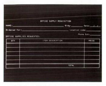
Fig. 2. Optional 2640A line drawing character set is used for grids, graphs, and pictorial information.
