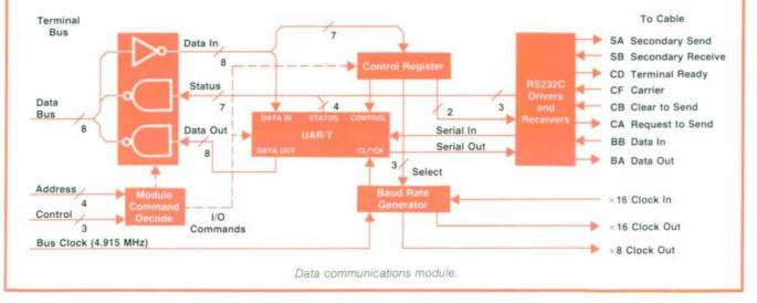
quires an interrupt. When the ATTENTION line of the terminal bus is low, indicating a processor interrupt request, the restart instruction causes a subroutine call to a special program to handle the needs of the data communications module. If ATTENTION is not set, the restart is changed to a no-operation and the program continues.
