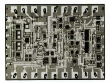
Fig. 4. Hybrid output stage uses discrete chips for drivers.
