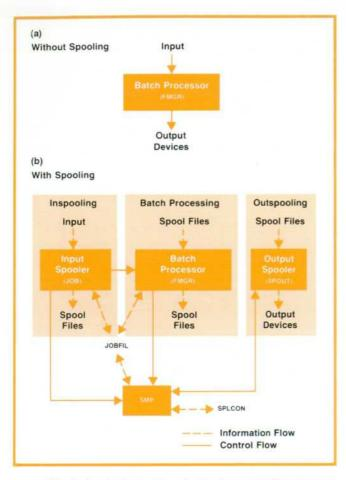
**Fig. 6.** Input/output with and without spooling. To use spooling, the user runs JOB instead of FMGR. JOB writes input to spool files on the disc and stores their locations and priorities in JOBFIL. FMGR then processes the jobs according to priority. SMP monitors the spool files, maintains an outspool queue (in SPLCON) for each device, and sends instructions to SPOUT, the output program.
