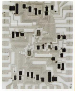
The small-sized precision resistors were realized by refining laser trimming techniques to work with smaller geometries. The number of probing pads was reduced by connecting selected resistors to common nodes with shorting tabs and opening the tabs with the laser after the resistors have been trimmed. The need for discrete chip capacitors was eliminated by using thick-film capacitors constructed with an interdigitated structure coated with a glass frit that has a high dielectric constant.
