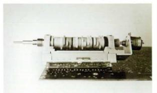
Besides contributing to a more visible mechanical layout, the plug-together design also simplified some of the circuits. By eliminating the cable-to-cable variations in adjacent lead capacitance, the plug-together construction permitted a reduction in the number of adjustments that would otherwise be required to normalize performance. The plug-together-by-function design also permits thorough testing of the individual circuit functions before final assembly.
