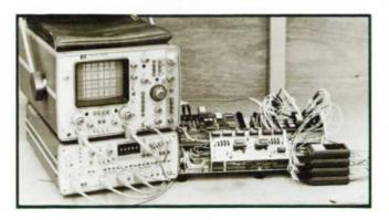
Fig. 3. Model 1740A Oscilloscope equipped with the logicstate option (opt 101) is available with Model 1607A Logic State Analyzer (lower unit) in a package known as Model 1740S.
