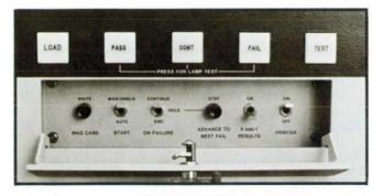
Fig. 5. The v AND I RESULTS switch causes the tester to vary the voltage and current on failed pins until the device passes and then print those voltage and current readings. See Fig. 6.
