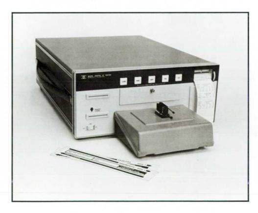
Fig. 1. Model 5045A Digital IC Tester is programmed by means of factory-prepared prerecorded magnetic cards to test a wide variety of commercially available digital integrated circuits. A builtin printer provides a record of test results and failure analyses. most often taken: each circuit is tested functionally and its voltage and current parameters are checked.
