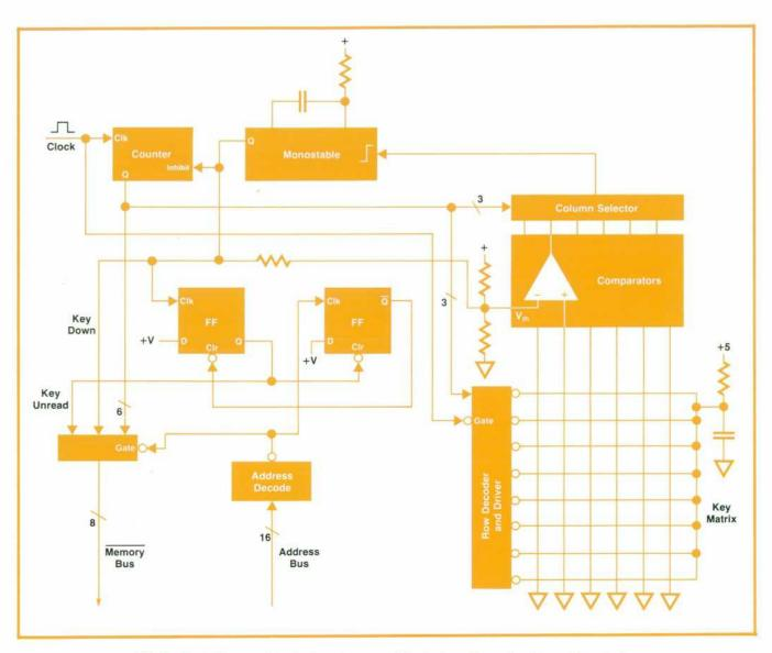
**Fig. 7.** Block diagram of the keyboard scanner. The keyboard is assigned an address in the instrument's memory and is read once every 160 μs. The two flags (KEY DOWN and KEY UNREAD) indicate to the instrument's microprocessor whether or not any action should be taken on the 6-bit key code presented to the memory bus.
