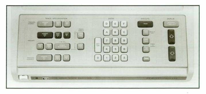
Fig. 1. Keys are grouped into four functional areas on the keyboard of the Model 1611A Logic State Analyzer. The keys that are most basic to instrument operation are in a darker shade.
