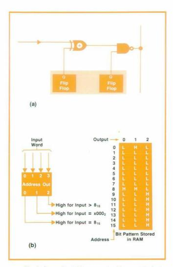
**Fig. 8.** Conventional bit comparator (a) separately implements storage of the reference bit, comparison, and enabling. Each bit in a word requires the circuitry shown here. A single RAM can be used as a multi-bit comparator (b) by loading the appropriate bit pattern (mask) into it, as shown by the table in this example.
