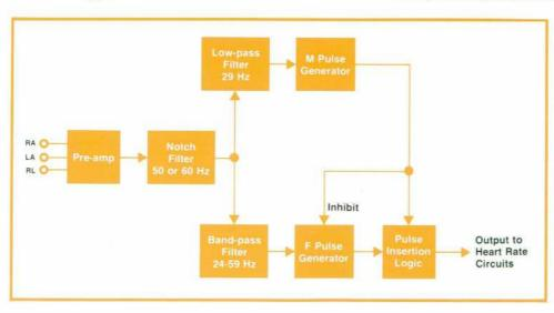
Fig. 5. Simplified block diagram of the AECG circuits. The basic scheme is to blank the F channel during a maternal ECG beat so the maternal ECG will not generate an F pulse. If blanking occurs at a time when an F pulse would have occurred, the logic circuits insert a pulse into the output stream.
