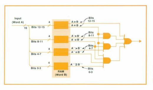
Fig. 9. A multi-bit comparator for wide digital numbers is implemented with relatively few components using the technique of Fig. 8b.
