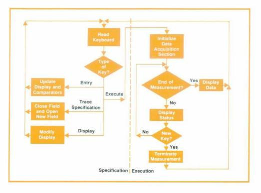
Fig. 4. Flow chart of firmware operation.
