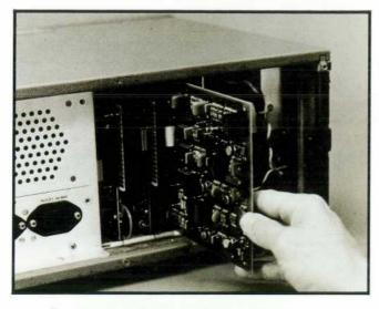
**Fig. 2.** Adding another monitoring technique to the Model 8030A Cardiotocograph is simply a matter of inserting a circuit card and then using the corresponding transducer. The instrument automatically makes the necessary circuit connections for whatever transducer is in use.
