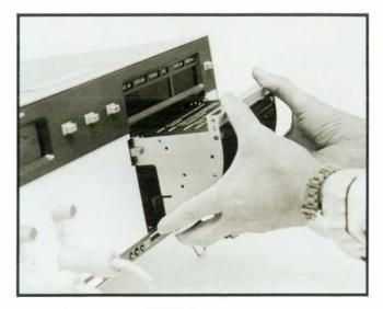
Fig. 3. Swinging the paper table up to the horizontal position allows the paper magazine to be withdrawn for easy loading.
