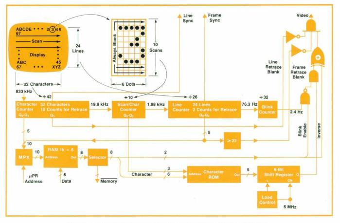
Fig. 10. Simplified diagram of the display logic for Model 1611 Logic State Analyzer.
