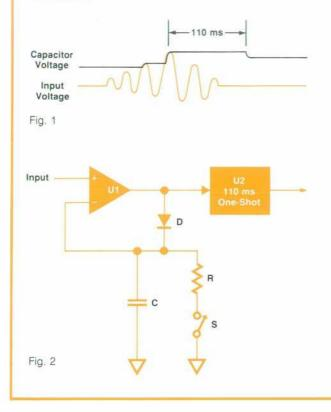
The circuit shown in Fig. 2 does this by storing the maximum level of each peak for 110 ms or until a higher peak occurs, whichever occurs first. A heart beat is indicated only when a maximum is held for 110 ms.
