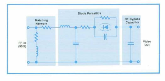
Fig. 4. Schematic representation of a low-barrier Schottky-diode detector.
