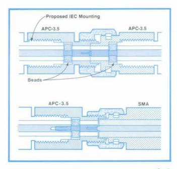
**Fig. 2.** A cross-section of mated male and female APC-3.5 connectors is shown in the upper drawing. The structure at the mating surface is an air-dielectric line with only the dimensions of the center and outer connectors controlling the impedance. The lower drawing shows how the APC-3.5 interfaces with the widely-used SMA connector.
