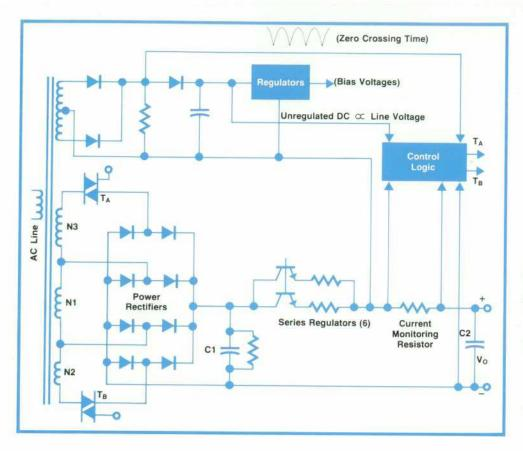
**Fig. 3.** Simplified diagram of Model 6002A's power circuits. The control logic monitors the output voltage, output current, and the line voltage level to decide which triacs ( $T_A$  and  $T_B$ ) should or should not be fired to connect the appropriate transformer taps to the power rectifiers (triacs are bipolar switches that conduct current in either direction if a gate pulse is properly applied and continue to conduct until the current from the source goes to zero).
