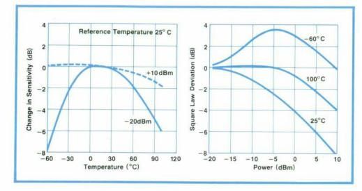
Fig. 5. The effects of temperature on the performance of a lowbarrier Schottky-diode detector (Model 33330C) when operating with a 10-k $\Omega$  video load. Detector performance is affected by the video load and the power level so for a given operating point, the effects of temperature can be minimized by the choice of load.
