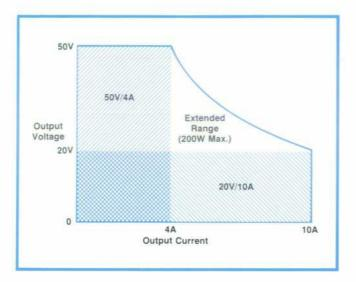
**Fig. 1.** Maximum output capability of Model 6002A DC Power Supply is bounded by 50 volts, 10 amperes, and 200 watts. At least three traditional 200W series-regulated power supplies would be required to cover the same range of output voltagecurrent combinations.
