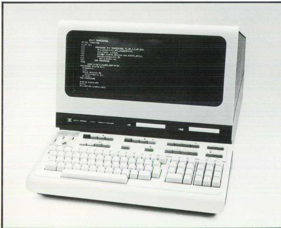
Fig. 1. Model 2641A APL Display Station is designed to serve as the principal user interface for APL \3000 and other APL systems. It has both APL and ASCII modes of operation.
