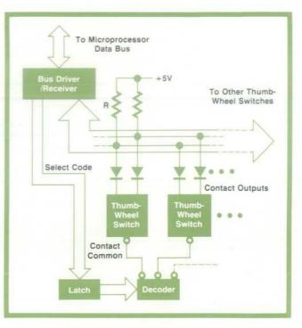
Fig. 6. Comparator option requires little hardware because of the capabilities provided by the microprocessor.
