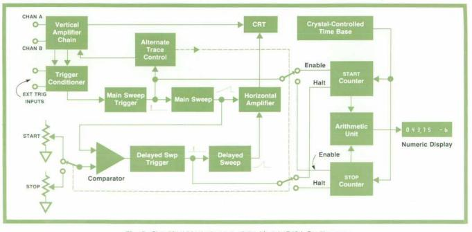
Fig. 5. Simplified block diagram of the Model 1743A Oscilloscope.
