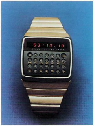
point has not been explicitly entered unless and until a colon or slash is entered in the display. The HP-01 is not a scientific calculator, so there is no enterexponent key. The range of decimal numbers that can be entered from the keyboard is .0000001 to 9999999., but display of results covers a greater range (this will be described shortly). Entry of leading zeros or multi-
