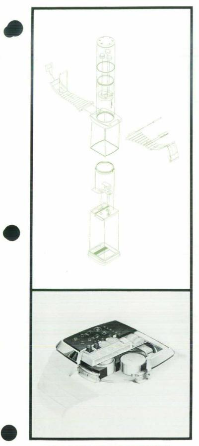
Fig. 4. Exploded and cutaway views of the HP-01.
