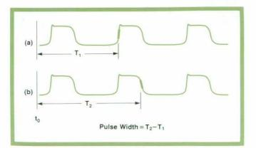
**Fig. 2.** Model 1743A Oscilloscope alternately measures the time from the start of the sweep to a point selected by the START control (a) and to a second point selected by the STOP control (b). Obtaining the difference between the two readings gives the time between START and STOP points.
