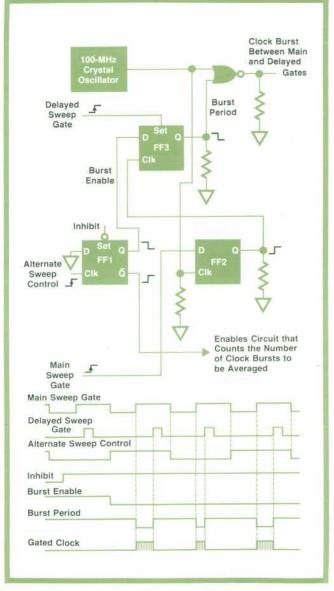
Fig. 7. Measurement-enable circuit generates bursts of clock pulses that extend from the start of the main sweep to the start of the delayed sweep. The start of each burst is synchronized to the clock pulses.
