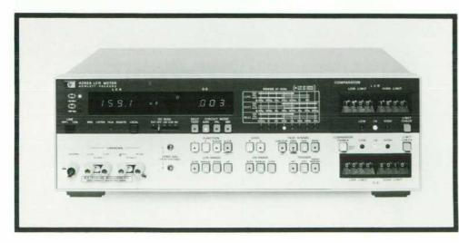
Fig. 1. Model 4262A LCR Meter, shown here with the comparator option installed, measures the inductance (L), capacitance (C), resistance (R), dissipation factor (D), and quality factor (Q) of components with 3½ digit resolution. Three test frequencies (120 Hz, 1 kHz, and 10 kHz) enable measurements of a wide range of component values.
