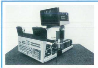
Fig. 3. Using a specially developed set of brackets and extenders, the computer can be serviced while fully operational.
