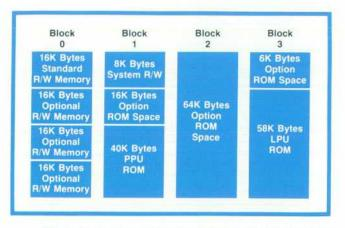
Fig. 2. System 45's 256K bytes of memory are partitioned into four blocks of 64K bytes each.
