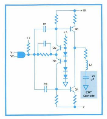
Fig. 9. High-speed video driver has fast rise and fall times, thereby assuring uniform brightness for both single dots and horizontal lines in spite of the 21-MHz display clock rate.
