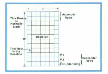
**Fig. 4.** Characters are formed in a basic  $5 \times 7$ -dot matrix contained in a field of  $7 \times 12$ -dots. Two columns of dots between each character are not used in the alphanumeric mode, but are used in the graphics mode to form continuous plots.
