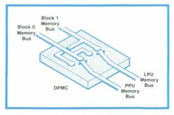
Fig. 4. Dual-port memory control (DPMC) coordinates memory accesses by the two processors. When the LPU and the PPU must communicate with the same block of memory the DPMC switches between them at a 50% duty cycle.
