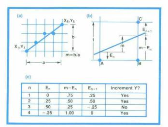
**Fig. 12.** Vectors are the basic elements of the graphics display. A vector is represented by series of dots on the CRT screen. Using a simple, fast dot-address algorithm, the PPU calculates the addresses of the dots that make up a vector, based on user-supplied end points. In the first octant, for each successive dot, the X value increments by one. The Y value may or may not increment, depending on the slope m and the error  $E_p$ .
