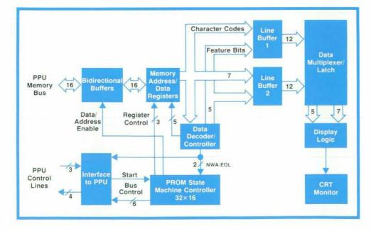
Fig. 10. Alphanumeric display block diagram.
