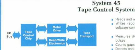
Fig. 1. System 45 tape control system. The tape control chip is a new 14,000-transistor NMOS design.
