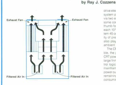
Fig. 1. Dual-fan parallel cooling scheme contributes to System 45's high degree of integration, as well as to reliability.
