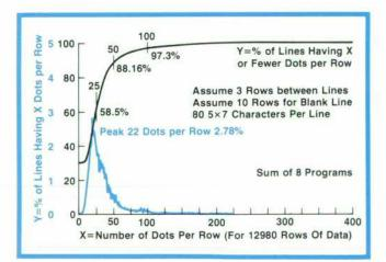
Fig. 5 Results of a study of the number of dots per row in a typical listing shows that 88% of the rows have 50 dots or fewer. To reduce peak power demand, the printer is designed to burn at most 56 dots at a time. Thus a complete 560-dot line takes ten burn sequences.
