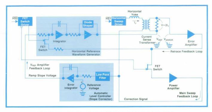
Fig. 7. System 45 horizontal sweep circuit uses active linearity correction. The scheme is frequency independent, thus allowing the use of two different horizontal frequencies for the alphanumeric and graphics rasters. The actual yoke current is compared with an ideal waveform to generate a correction signal.
