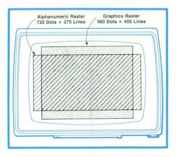
Fig. 6. Dual raster scan circuitry was developed for the CRT display so the size and aspect ratio of the displayed information could be optimized for both alphanumerics and graphics.
