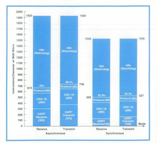
Fig. 4. Multipoint card microprocessor timing load at 9600 bits per second, the fastest terminal rate. The microprocessor can execute 1920 instructions in the time it takes to receive or transmit each ten-bit asynchronous character at this rate. Eight-bit synchronous characters take less time, enough for 1536 instructions. In either case the microprocessor idles much of the time.
