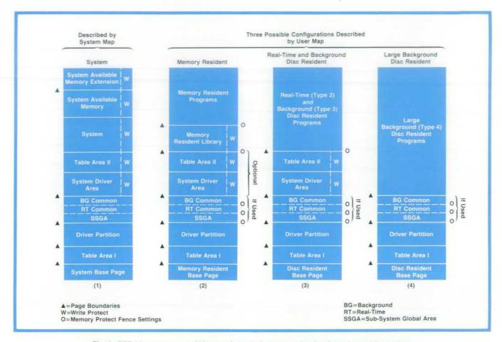
**Fig. 1.** RTE-IV manages up to 2M bytes of physical memory using the dynamic mapping system, a hardware option to HP 1000 Computers. Segments of physical memory are mapped into 64K-byte logical memory spaces according to four maps: the system map, the user map, and two dual-channel port controller maps. At left is a picture of the system map as it would look when processing an interrupt. Also shown are three possible user map configurations. The maps are set up by the operating system.
