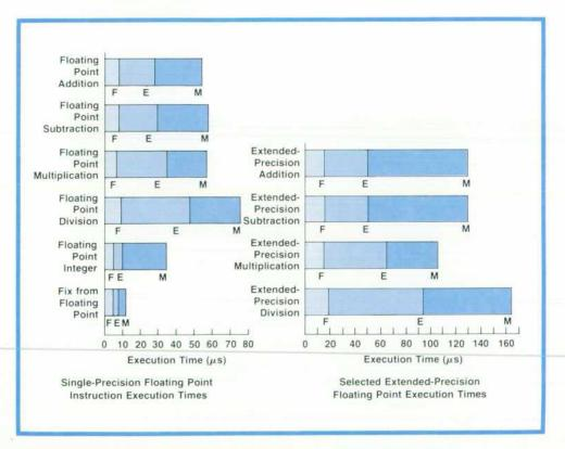
Fig. 2. Execution times of floating point instructions on the M-Series, the E-Series, and the new F-Series. HP 1000 Computers. The E-Series has a faster CPU than the M-Series. The F-Series has a hardware floating point processor and the same CPU as the E-Series.
