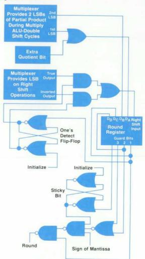
**Fig. 1.** Floating point processor rounding circuits. Depending on the operation, rounding information is set up in the round register in four ways: the least significant bit may be shifted into the round register through a multiplexer, subtrahend bits may be complemented as they are shifted into the round register, two partial product bits may be loaded into the round register, or a quotient bit may be loaded into the first guard bit of the round register.
