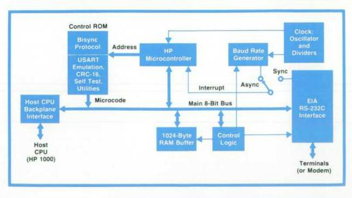
Fig. 3. Multipoint interface card performs three main functions: USART (universal synchronous/ asynchronous receiver/transmitter), multipoint protocol, and error control.
