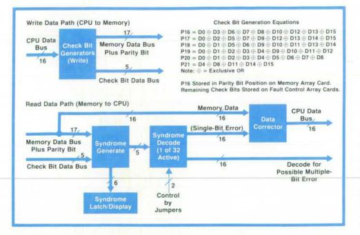
Fig. 3. Fault control memory generates and stores six check bits (P16-P21) on each write to memory. On each read from memory, the six check bits are regenerated from the data bits (D0-D15) and compared with the stored check bits to form a two-octal-digit syndrome that indicates the type of error, if any. Single-digit errors are automatically corrected by inverting the erroneous bit.
