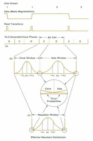
Fig. 7. Flexible disc drives divide each bit cell into a clock window and a data window. Lower curves show probability distributions for the locations of bit transitions within these windows. Errors occur if any transition falls outside its intended window.
