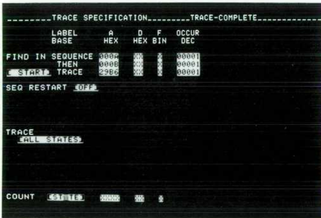
Fig. 3. Menu display fields (highlighted by inverse video) that may be changed by the keyboard in setting up instrument controls. The menu shown here tells the analyzer it must first find state 000A and then 000B in that order before allowing state 29B6 to start data capture.
