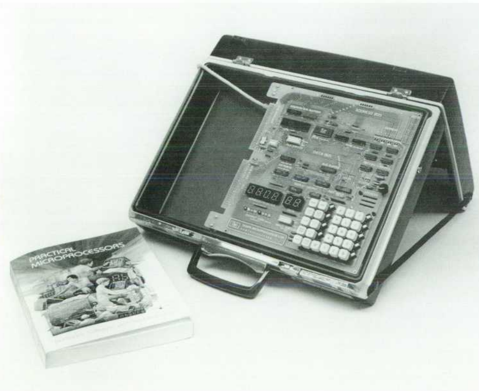
Fig. 1. Model 5036A Microprocessor Lab includes a keyboard-controlled microcomputer and a comprehensive textbook that contains both text and experiments.
