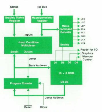
Fig. 3. Block diagram of graphics controller.
