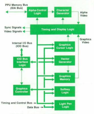
Fig. 2. Block diagram of graphics system.
