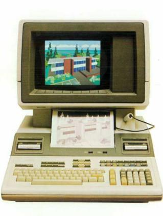
Fig. 2. The System 45C is an integrated computer graphics system with a high-resolution color display, thermal printer, two tape cartridge drives, light pen, high-performance I/O, and mass storage capability.
