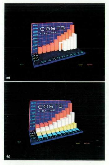
**Fig. 10.** Dominant area fill simplifies hidden surface removal for the generation of 3-D images. The bar chart started in (a) uses dominant area fill to achieve the final result shown by (b). As the chart is constructed from the back, the columns in front replace those areas immediately behind the columns.
