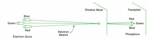
Fig.1. Three electron guns are arranged in a triangular pattern in the neck of the color CRT. The beams from these guns all pass through a single hole in the shadow mask to excite a triangular arrangement of red, blue, and green phosphor dots on the faceplate.
