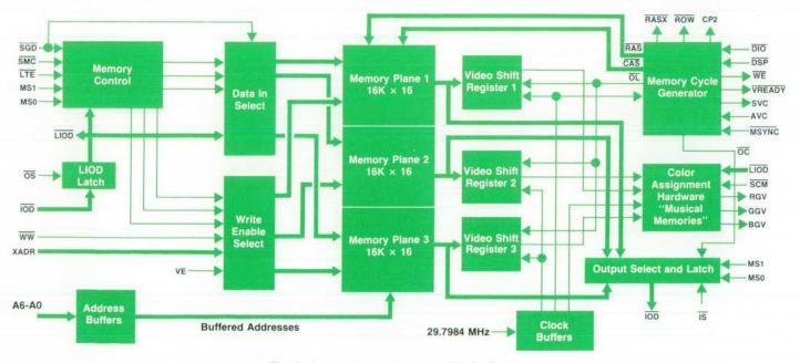
Fig. 5. Graphics memory system block diagram.
