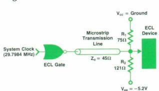
Fig. 2. Microstrip transmission lines are used to transmit clock signals over distances greater than five to eight centimetres. This minimizes reflections and maintains signal integrity.
