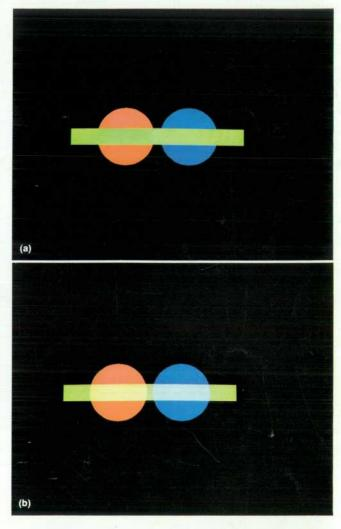
**Fig. 11.** In (a) dominant area fill gives the result shown when a green rectangle is plotted over the red and blue circles. However, if the area fill is nondominant, the green area is modified by the previous background colors as depicted in (b).
