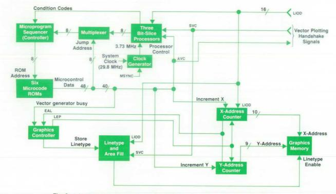
Fig. 8. A bit-slice processor system in the 9845C replaces the vector-generation firmware algorithm used in the 9845A/B. This approach makes the vector generation rate up to 50 times faster than for earlier 9845 Computers.
