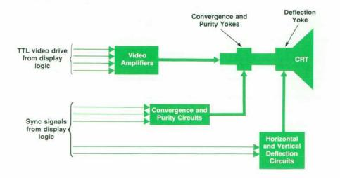
Fig. 2. Block diagram of drive circuits for the System 45C color CRT.
