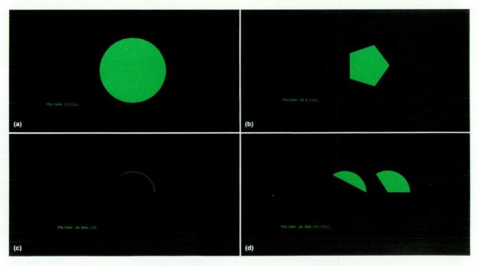
**Fig. 3.** (a) Circle drawn and filled by the POLYGON 15, FILL statement using the default value of 60 sides for the polygon. (b) Pentagon drawn and filled by the POLYGON 10, 5, FILL statement. (c) Arc drawn by the POLYGON 10, 360, 122 statement. (d) When the FILL declarative is added to the statement in (c), the shapes shown are obtained for the two cases where the pen is up or down prior to execution. The area-fill algorithm connects the first and last points of a line to fill in an area.
