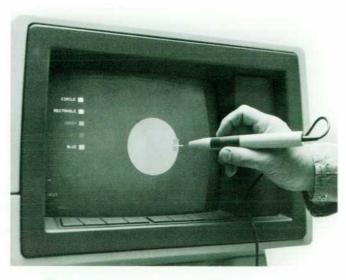
Fig. 1. The System 45C light pen can be used to pick displayed objects or menu items and to place objects or indicate dimensions.
