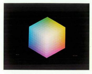
Fig. 1. Color cube model. Area-fill colors can be specified by selecting a point within this unit cube. The three coordinates for the point indicate the fractions of red, blue, and green required for the specified color.
