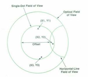
Fig. 4. Relationship between the shapes and locations of the single-dot and horizontal-line fields of view. The horizontal offset is caused by the higher threshold level for a horizontal line as shown in Fig. 3b and by the detection circuit delays.
