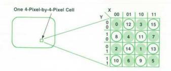
**Fig. 9.** Area fill colors are obtained by varying the pattern in 4 × 4 arrays of pixels. These patterns are generated in response to the parameters specified by the AREA COLOR or AREA IN-TENSITY statements.
