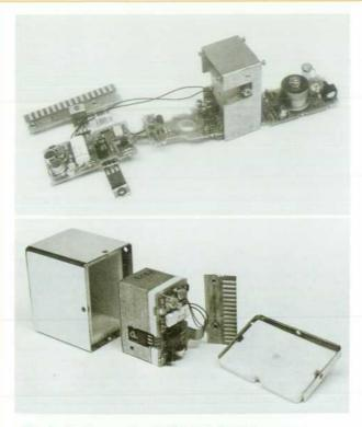
Fig. 3. Final assembly of 10811A/B Oscillator.
