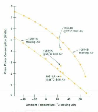
Fig. 4. Steady-state oven power of the 10811A compared with that of the 10544A/B.
