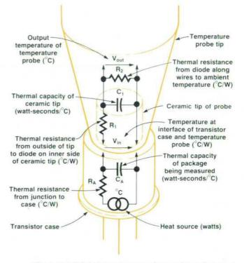
Fig. 2. Simplified electrical analog of the problem of measuring the temperature of a transistor with a probe.
