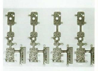
Fig. 2. Flex circuits come five to a panel and are loaded, soldered, and tested before being separated.
