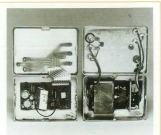
Fig. 4. The sculptured flexible circuit interconnect of the 10811B (left) is a significant improvement over the older 10544C (right).
