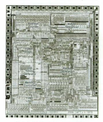
Fig. 3. Photomicrograph of the video control chip.
