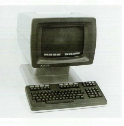
Fig. 1. Model 2626A Display Station is a multi-workspace, multiwindow computer terminal that has dual data communications ports. Its capabilities may be configured dynamically as four logically independent virtual terminals. The terminal can handle line lengths up to 160 characters and offers foreign language options and an optional built-in printer. it is almost totally left to the user.
