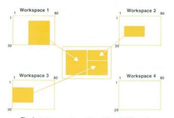
Fig. 2. In this example, portions of three 2626A workspaces are displayed in windows on the screen. Workspace 4 is not displayed. of softkey levels having similar functions.
