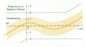
Fig. 4. Typical 10023A error curve with possible unit-to-unit variations (shaded band).
