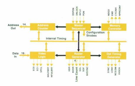
Fig. 1. Block diagram of the video control chip (VCC). Several interlocked state machines and counters are driven by parameters read from the display memory (black lines are control paths).
