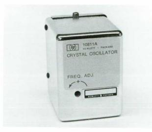
Fig. 1. The new 10811A/B 10-MHz Crystal Oscillator is a component oscillator for instruments and systems. A new quartz crystal cut and a new circuit design give it many improved features including lower phase noise and lower power consumption than previous designs. Two models, A and B, provide a choice of electrical connection methods.
