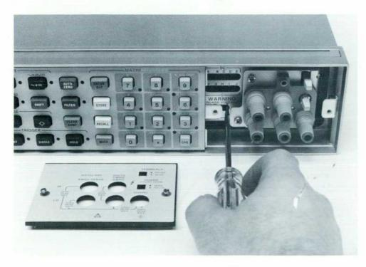
Fig. 14. All functions and ranges of the 3456A DVM can be completely calibrated from the front panel of the instrument by removing the cover at the right as shown.
