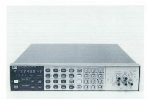
**Fig. 1.** The HP Model 3456A Digital Voltmeter is a 3½to-6½digit, fully-guarded integrating voltmeter with flexibility and precision, designed for both bench and system measurement applications.
