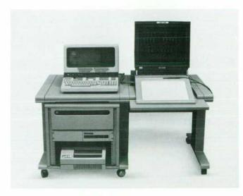
Fig. 1. IGS workstation consists of computer, CRT terminal, graphics tablet, and high-resolution color display.
