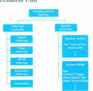
Fig. 1. Firmware organization of the 3497A Data Acquisition/Control Unit.
