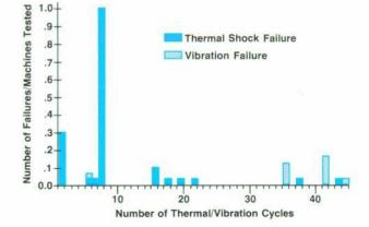
Fig. 1. Failure rate versus number of thermal and vibration cycles. The data shows that most of the units failed during the seventh thermal cycle and that most vibration-induced failures occurred later in the strife testing.
