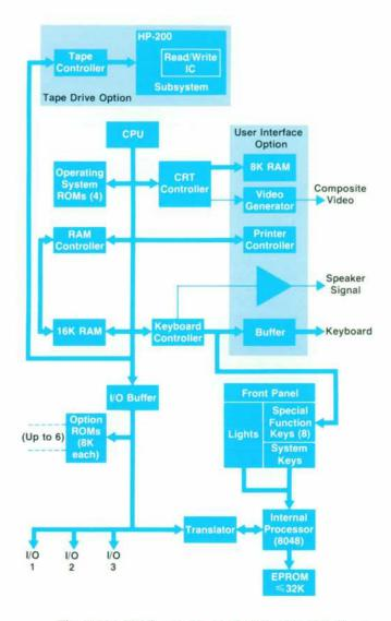
Fig. 2. The 9915A uses the architecture of the HP-85 partitioned as shown in the above block diagram.
