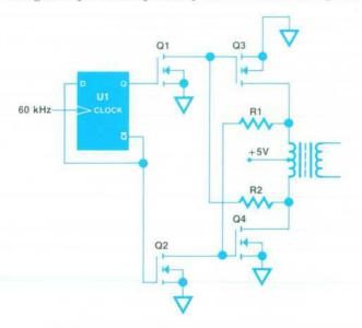
Fig. 5. Simplified schematic of the dc-to-dc converter power supply used in the voltage and current D-to-A plug-ins. 3497A since each digital input plug-in handles up to eight interrupts and up to five such plug-ins can be inserted in the 3497A. This method uses the counter output line as an interrupt line that changes level whenever a measurement is completed or an overflow occurs.
