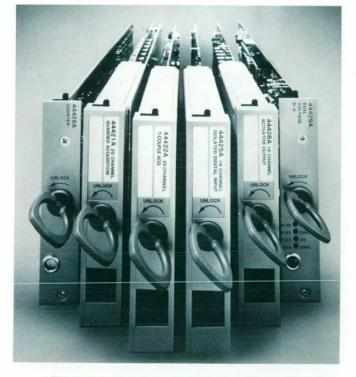
Fig. 1. The 3497A Data Acquisition/Control Unit has a variety of plug-in assemblies that measure physical parameters, actuate devices, input and output digital data, convert digital commands to voltages and currents, and scan many channels.
