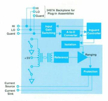
Fig. 5. Block diagram of 3497A voltmeter module.
