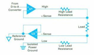
Fig. 6. Output stage and remote sense connections for voltage D-to-A converter plug-in.
