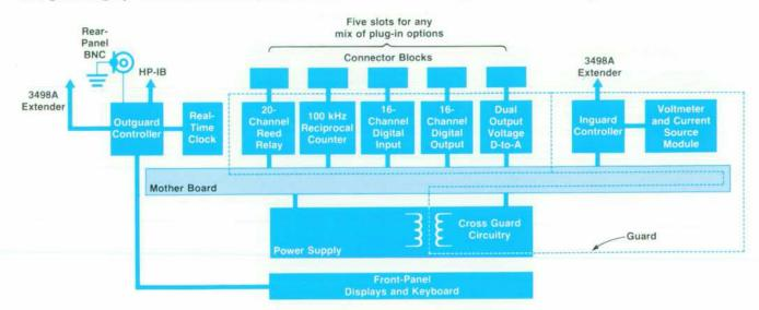
Fig. 4. Block diagram of the 3497A Data Acquisition/Control Unit.
