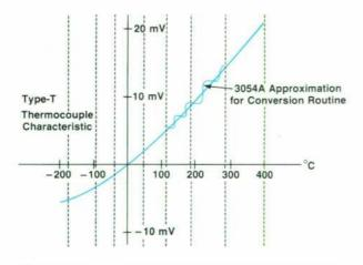
Fig. 1. The 3054A conversion routines divide a thermocouple characteristic into eight unequal temperature intervals so that third-order polynomials can be used within each interval to approximate the curve with about equal error.
