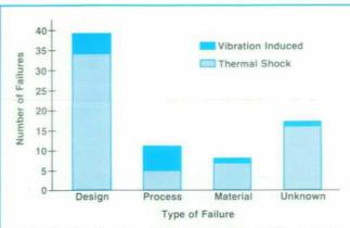
Fig. 3. Classification of failure types induced by thermal shock and by vibration (a total of 63 thermal shock and 13 vibration failures during initial strife testing of 40 units).
