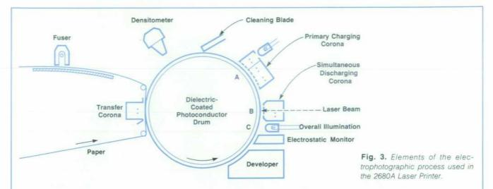
toner along with larger iron-based particles known as carrier. This toner is transported to the drum on a magnetic brush which generates a toner cloud at the drum surface. The toner is charged in such a way that it is attracted to the portions of the drum near zero volts and is not attracted to the portions of the drum surface with a high positive potential. There is now a visible image on the surface of the drum, with toner in the areas that were exposed by the laser beam.
