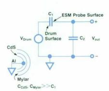
Fig. 1. Electrostatic monitor (ESM) equivalent circuit. The ESM is a noncontacting electrostatic voltmeter used to measure drum potentials.
