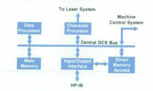
Fig. 1. Block diagram of the data control system of the 2680A Laser Printer.
