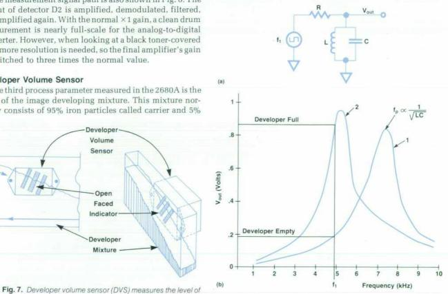
Fig. 8. DVS circuit and frequency response.
