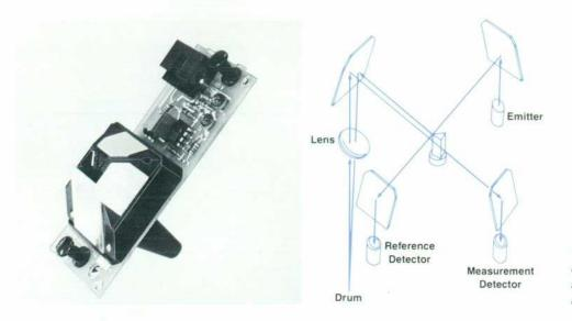
Fig. 5. Density monitor (DSM) measures developed image density by reflecting infrared light from a process mark on the drum.
