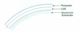
Fig. 1. Photoconductor drum construction.
