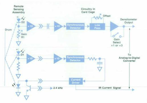
with time; for the same drive current, the light output drops. This would directly affect the density measurement, but with closed-loop control of the drive current, the light output remains calibrated after the gain is set by R1 in Fig. 6. A signal from the current driver is used to determine if the current is within an acceptable range.
