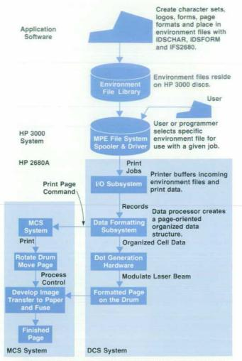
Fig. 1. Architecture of the HP 2680 Laser Printing System.
