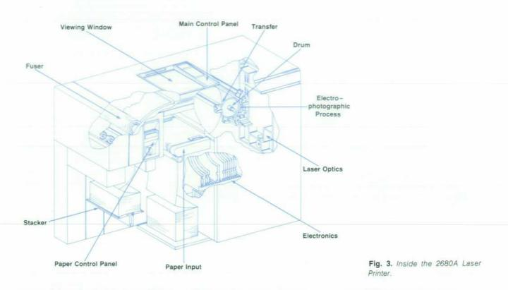
photoconductor drum to the paper. The printed image can be viewed by the operator at the viewing window. The paper then passes through the fuser system, where the printed output is permanently fixed to the paper. Finally, the paper is folded and stacked by the stacker. Operation of the paper system (threading, splicing, stacking, etc.) is controlled by the paper control panel. The overall print process and printer diagnostic routines are controlled by the main control panel.
