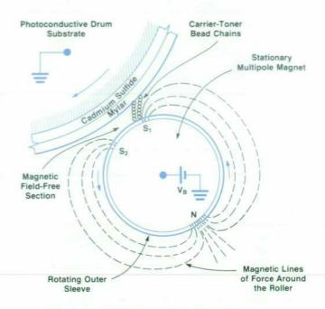
Fig. 1. Toner developing unit configuration.
