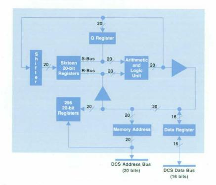
Fig. 2. Data processor data paths.
