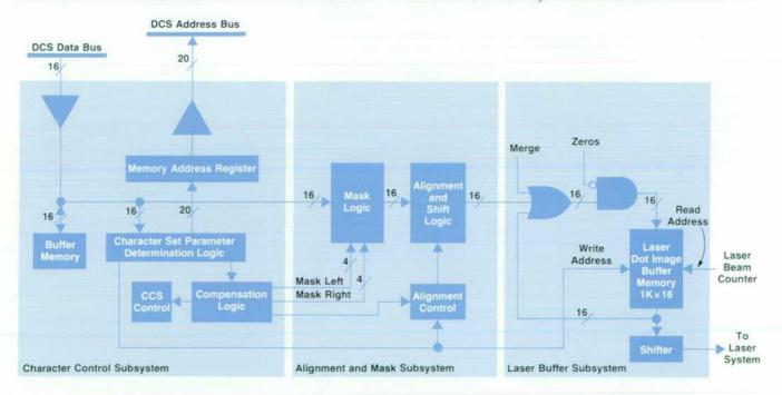
Fig. 3. Character processor block diagram.
