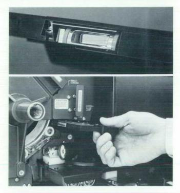
Fig. 4. ESM probe assembly and mounting location.
