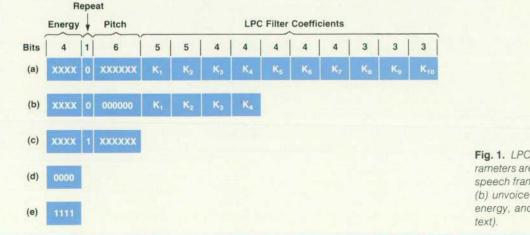
Fig. 1. LPC speech synthesis parameters are stored into one of five speech frame formats: (a) voiced, (b) unvoiced, (c) repeat, (d) zero energy, and (e) stop frames (see text).
