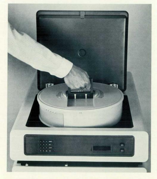
Fig. 2. The HP 97935A Data Pack for the 7935 Disc Drive provides contamination resistance similar to a sealed chamber. When the pack is inserted in the filtered air of the drive, a trap door opens to allow the heads access to the media. this data movement as well as the subsequent skipping of the defects in a manner that is transparent to the host computer.
