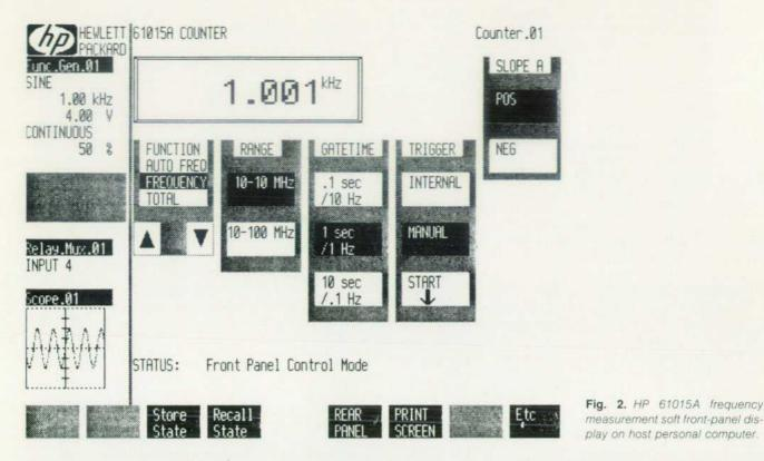
the prescaler is invoked and only two gate times are available (0.1 s for 10-Hz resolution and 1 s for 1-Hz resolution). This illustrates the "you see only what you can control" philosophy of the PC Instruments soft front-panel application software. The autofrequency measurement (Fig. 3) is the most striking example of this minimum display philosophy as applied to the HP 61015A.
