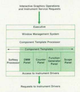
Fig. 7. Soft front-panel architecture. Shaded areas are instrument-specific functions.
