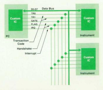
Fig. 2. PCIB parallel communications channel.
