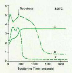
Fig. 5. SIMS profiles of boron, fluorine, and silicon in the silicon substrate and titanium silicide layers after isochronal annealing in a vacuum.
