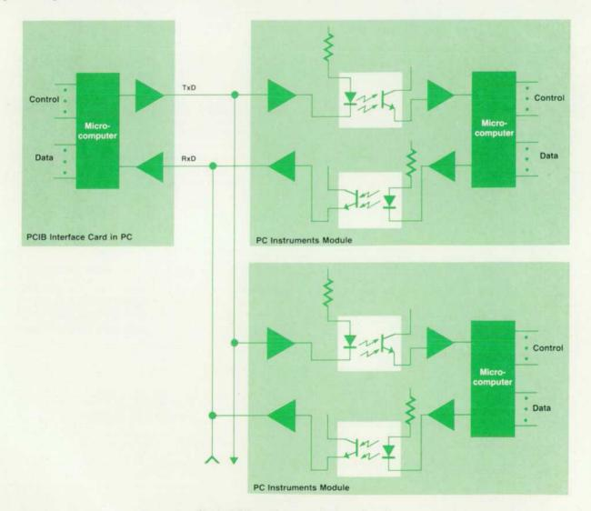
Fig. 3. PCIB serial communications channel.
