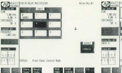
Fig. 5. Example of ganged switch (Input block at upper left center) from HP 61011A Relay Multiplexer module for PC Instruments.
