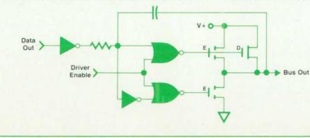
Fig. 1. Simplified block diagram of the controlled rise-fall PCIB predriver and output driver. Bootstrapping circuitry is not shown.
