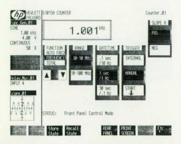
Fig. 9. Counter soft front-panel display in frequency mode.
