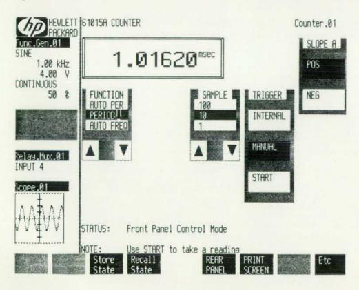
Fig. 10. Counter soft front-panel display in period mode.
