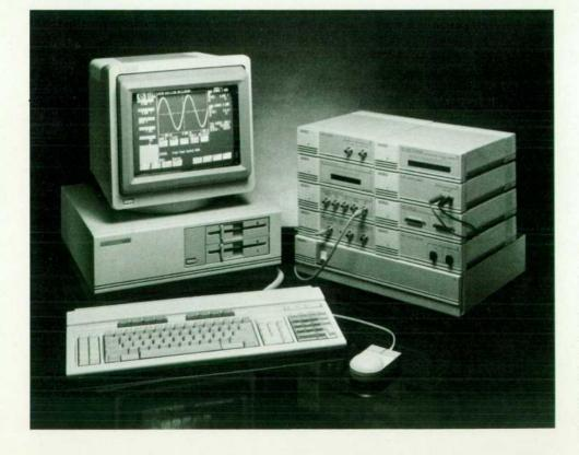
Fig. 1. The HP PC Instruments system is designed to work in concert with the HP Vectra and HP 150 Computers and the IBM PC/ XT/AT computers. Eight different instruments, offered in modular, stackable cases, and several software packages and accessories are available. A single interface card will support any combination of up to eight modules. More instruments can be added by using additional interface cards.
