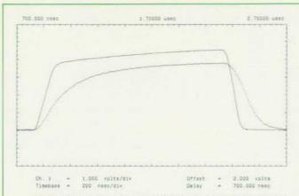
Fig. 2. Difference in rise and fall times (room temperature) for a 10:1 ratio of capacitive load, same custom IC and axis scaling. Capacitance varies from 130 pF to 1.3 nF. Actual pulse widths on the PCIB are much longer.
