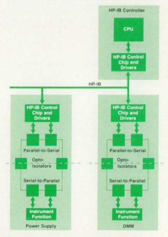
Fig. 1. Typical HP-IB system with isolated instruments.
