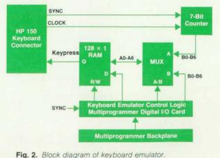
seven-bit binary counter clocked by the standard keyboard pulses from the HP 150 sequences through the RAM locations. A keypress signal is returned when the counter addresses the RAM location that was programmed to be sent. The HP 150 determines which key is pressed by keeping track of the clock pulses it had to send before it received the keypress signal.
