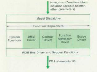
Fig. 3. Instrument driver architecture. Shaded areas are instrument specific functions.
