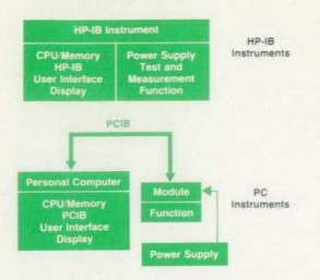
Fig. 2. Difference in HP-IB and PCIB architectures.
