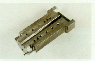
Fig. 4. A special taper (left) in the waveguide (right) acts as a 37-GHz high-pass filter and 4:1 impedance transformer. The taper is formed by numerically controlled milling machines according to equations describing the taper's dimensions.
