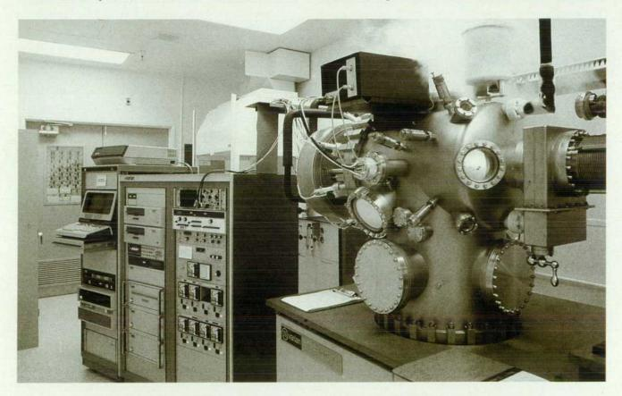
Fig. 3. HP's MBE systems (right) are controlled by HP 1000 Computers (left).
