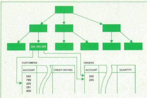
(205). The pointer associated with this key value points to the tuple in the relation that contains this same value. Each tuple in the relation is pointed to by one and only one entry in a leaf page of the index.
