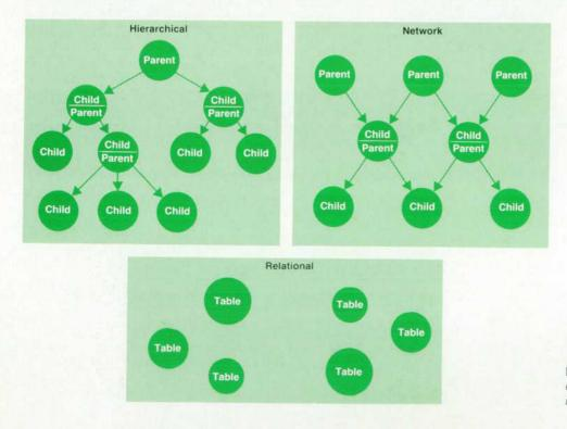
Fig. 1. The three data base models used by data base management systems. ware to define their own access order. It is this variety of access structures that enables DBCore to support both network and relational data base models.
