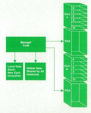
Fig. 13. An instance of a manager is made up of four data areas.
