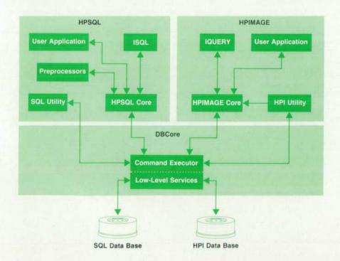
Fig. 2. HP ALLBASE product structure. HPSQL is the relational user interface. HPIMAGE is the network user interface. DBCore is used by both interfaces. (DML). The following scenario describes how the DBCore DML is invoked by the ALLBASE interfaces in a typical data base application.
