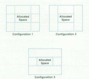
Fig. 7. Different memory allocation configurations possible when space for a box is allocated from a larger box.
