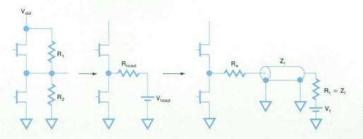
Fig. 13. Transformation of a desired load to resistive divider parameters.
