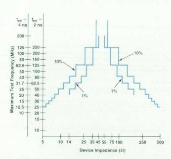
Fig. 5. Maximum test frequency in an unterminated environment. Any DUT switching time is assumed to be zero and any transition time is assumed to be zero.
