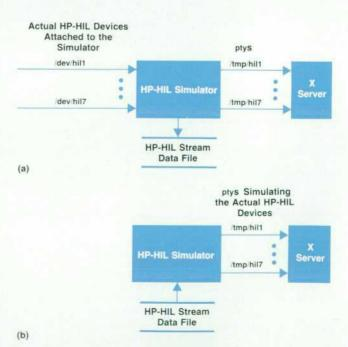
Fig. 2. (a) Initial setup for recording data from HP-HIL devices. (b) Setup for playback. fold. The simulator was also used by another group to simulate foreign versions of the HP-HIL keyboard to test native language support (NLS) functionality.
