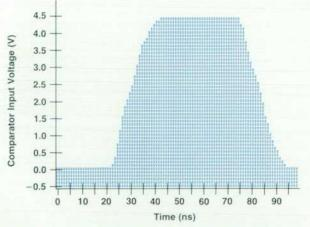
**Fig. 2.** Shmoo plot of comparator input signal from an HCMOS output buffer with 4-mA source/sink capability, loaded by an open-ended transmission line ( $t_{pd} = 3 \text{ ns}$ ) with the comparator in high-Z mode (lumped capacitance = 23 pF).
