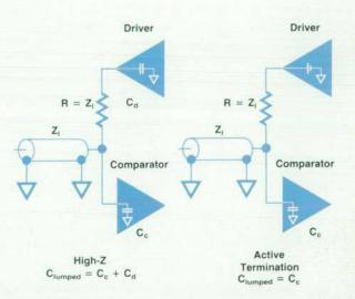
Fig. C. Operating modes of the receiver path.
