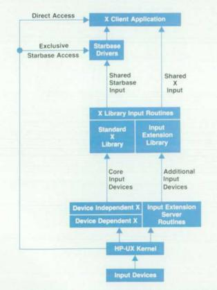
Fig. 1. Input data flow in the Starbase/X11 Merge X server.
