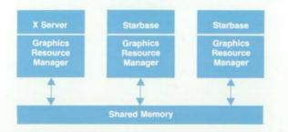
Fig. 4. Architecture for constructing the GRM as a library.
