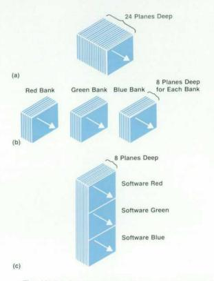
Fig. 12. (a) A 24-plane-deep window on the screen. Of course the physical depth of display memory is not seen by the user. (b) 24-plane-deep backing store in offscreen frame buffer memory organized in three hardware banks of 8 planes each. The picture on the display is replicated on the three banks. (c) 24-plane-deep backing store in virtual memory. This is a contiguous piece of memory organized in three compartments. Each compartment is a software bank mirroring the hardware banks.
