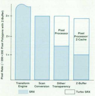
Fig. 3. Relative performance of 3D graphics pipeline stages for large polygons.
