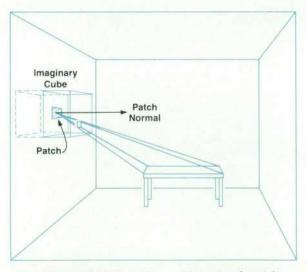
An imaginary cube is created around the center of a patch. Every other patch in the environment is projected onto the cube.
