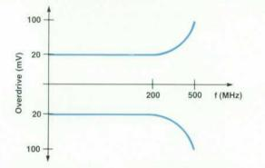
Fig. 15. Comparator overdrive as a function of data rate.
