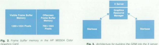
Fig. 3. Architecture for building the GRM into the X server.
