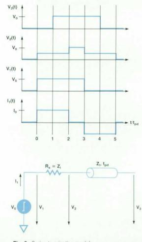
Fig. 3. Series termination model.
