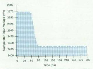
**Fig. 3.** CMOS MC14000 family output signal ( $V_{oh} = 2.5V$  at  $I_{oh} = 2.1 \text{ mA}$ ,  $V_{ol} = 0.4V$  at  $I_{ol} = 0.44 \text{ mA}$ ) with resistive divider parameters  $R_s = 1000\Omega$ ,  $V_t = 2.5V$ .
