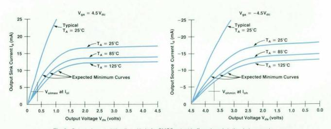
**Fig. 8.** Output characteristics ( $I_d$  vs  $V_{ds}$ ) of a CMOS output buffer, where  $I_d$  is the drain current and  $V_{ds}$  is the drain-to-source voltage across the FET.
