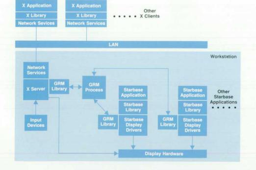
Fig. 3. Starbase/X11 Merge software architecture. /\* FillScanline is an XDI routine that accomplishes the fill request \*/
