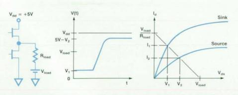
Fig. 10. CMOS output driving a resistive load.
