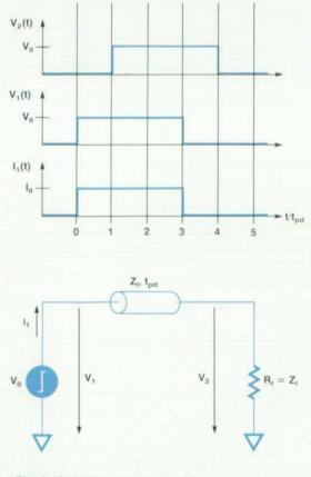
Fig. 2. Parallel termination model.
