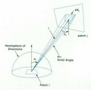
Fig. 6. The area dAj is taken to be the area of patch j that is visible through the solid angle  $d\omega$ . Adapted from Wallace.<sup>10</sup> Used with permission.
