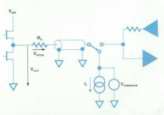
Fig. 17. Dc measurement path using the resistive divider.
