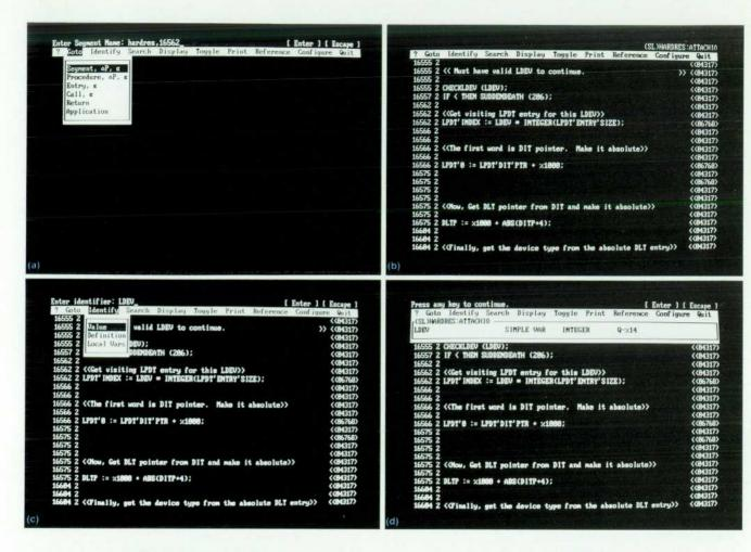
Fig. 5. Screens from a typical HP Source Reader session. (a) The GOTO SEGMENT HARDRES command is entered. (b) Resulting screen. (c) Invoking the IDENTIFY VALUE command. (d) Resulting screen.
