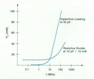
**Fig. 16.** Device under test power dissipation as a function of frequency for capacitive loading at 50 pF and for a resistive divider with 10-mW dc loading + 10-pF capacitance.
