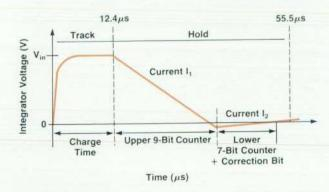
Fig. 6. Integrator voltage waveform for triple-slope integration.
