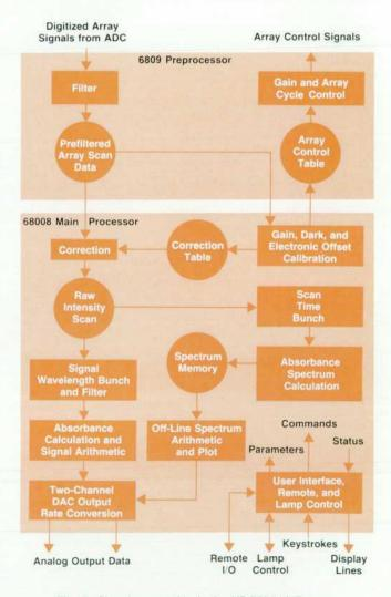
Fig. 8. Signal processing in the HP 79854A Detector.
