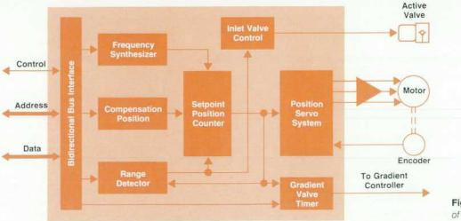
Fig. 4. Simplified block diagram of the pump control chip.
