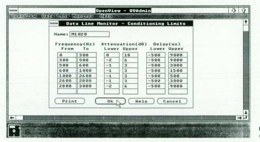
Fig. 3. Screen used to enter conditioning limits.
