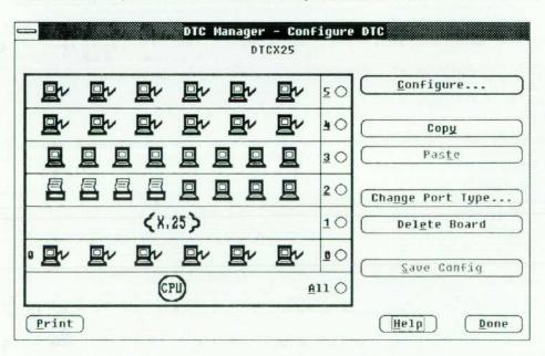
Fig. 1. Most HP OpenView DTC Manager functions begin with the display of the DTC rear panel, which shows the types of cards and devices that are plugged into the DTC. DTC stands for datacom and terminal controller. to trigger management functions on the local area network DTC components.
