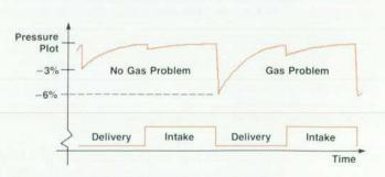
Fig. 15. Gas bubble detection using ripple information.
