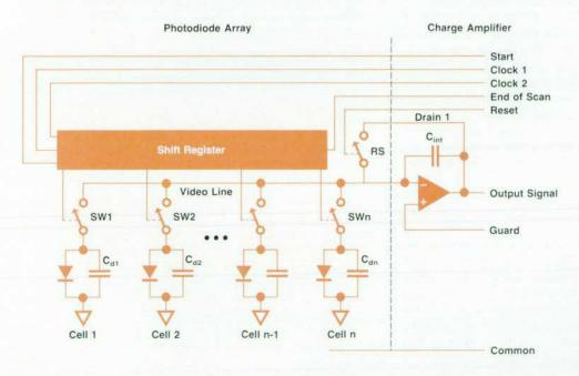
Fig. 5. Schematic diagram of a self-scanning photodiode array.
