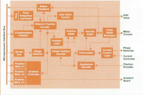
Fig. 1. Functional block diagram of the HP 1050 pump control chip.
