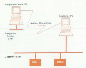
Fig. 4. The HP OpenView DTC manager allows remote access to all DTC functions. For example, from a PC in the HP Response Center an HP support engineer can access a customer's DTCs.
