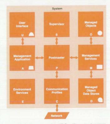
Fig. 4. Components of the HP OpenView network management architecture reference model.
