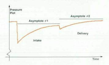
Fig. 17. An example of flow asymmetry caused by a leaky first piston.
