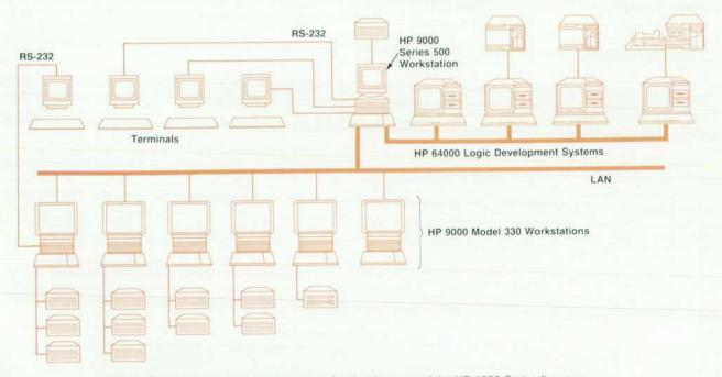
Fig. 3. Workstation and emulator network for development of the HP 1050 Series firmware.
