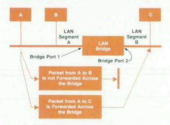
Fig. 1. How a LAN bridge isolates traffic.
