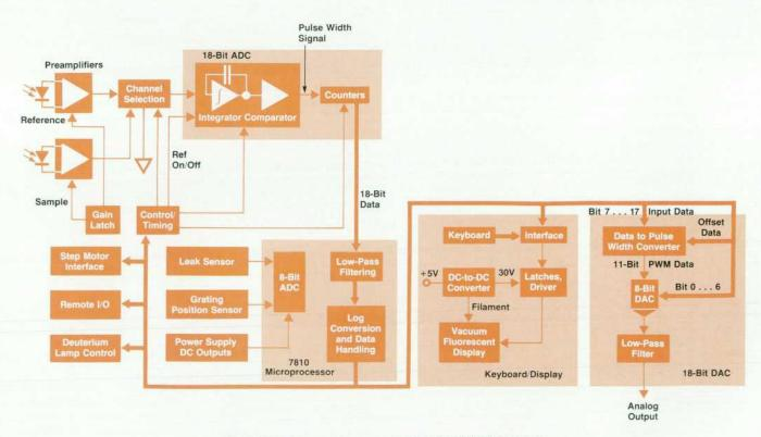
Fig. 3. Signal processing system of the HP 79853A Detector
