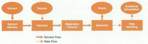
Fig. 1. Functional diagram for high-performance liquid chromatography (HPLC).
