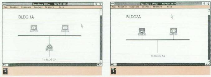
Fig. 3. Hierarchical network map. Note that the subnet symbol is used to depict the existence of network configurations in different buildings.
