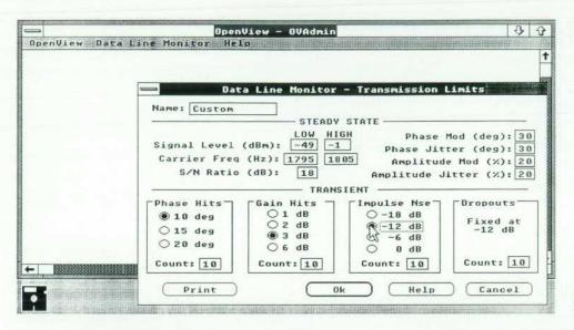
Fig. 2. Screen used to enter transmission limits.
