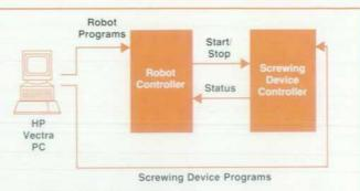
Fig. 4. Robot station data flow.
