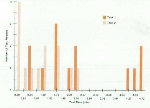
Fig. 10. Results of part three of the HP 1050 Series user friendliness test for the pump module. The large span of times required by the test persons for task 1 is significantly reduced for task 2, which was similar to task 1. This is an indication of the learnability of the product.
