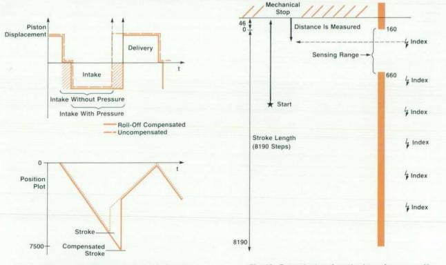
Fig. 9. Influence of lengthened stroke on intake volume.
