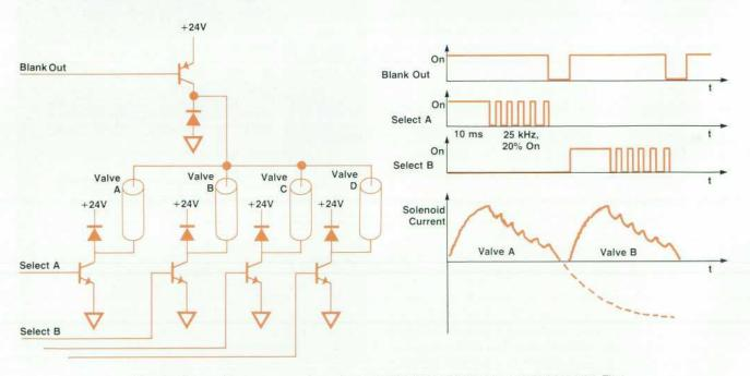
Fig. 12. Schematic diagram and waveforms for the inlet valve of the quaternary pump. The waveforms indicate transistor states, not voltage levels.
