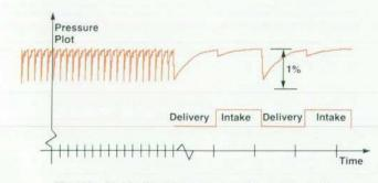
**Fig. 14.** A typical pressure trace and its relation to the pump cycle (right side time scale expanded).
