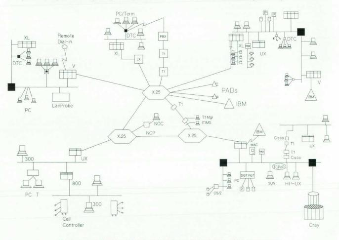
Fig. 1. Typical enterprise network includes both local and wide area netorking technologies and an assortment of network devices from different vendors.
