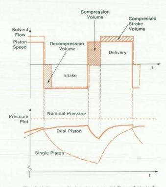
Fig. 6. Influence of solvent compressibility and elasticity.
