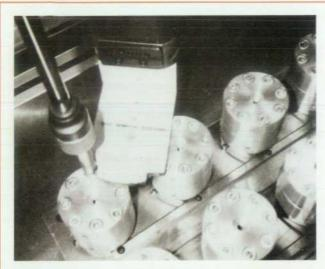
Fig. 3. Installing a damper screw.
