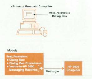
Fig. 4. The design strategy for modularization in OV/NSM/ Vectra for a particular user activity. The dialog box, the dialog box procedures, and the Vectra-to-HP 3000 routines are combined into one module.
