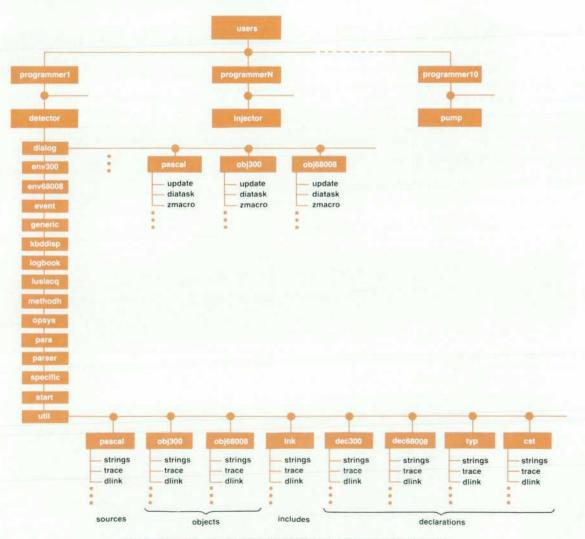
Fig. 4. Directory structure for HP 1050 Series firmware development.
