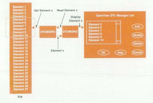
Fig. 9. HP OpenView DTC Manager lists are dialog boxes that contain list boxes that are managed by DTCMGRUI instead of Microsoft Windows. The items in the list are requested one by one from DTCMGRIO (through RL Switch). corresponding menu item in the Tools menu.
