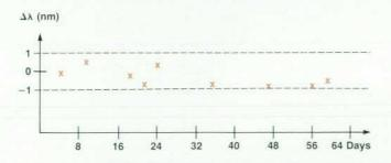
Fig. 3. Plot of the wavelength calibration accuracy of the HP 1050 Series diode array detector. The test time of 64 days corresponds to over two years of normal operation, assuming an acceleration factor of five and 3500 operating hours per year. tem levels, we do mainly the second type of strife testing.
