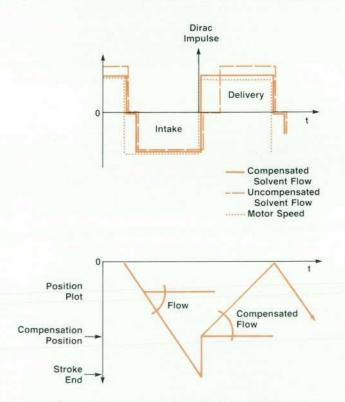
Fig. 7. Ripple compensation with compression jump.
