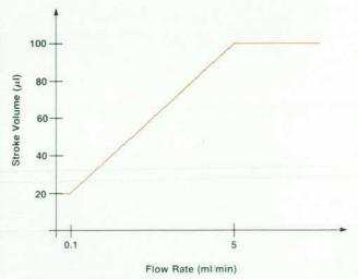
Fig. 2. Stroke volume as a function of flow rate, showing the variable stroke capability of the HP 1050 pump.
