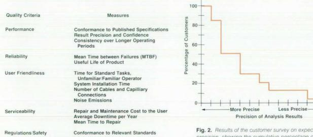
Fig. 1. Key quality criteria and measures applied to define and verify the quality of the HP 1050 Series LC system.
