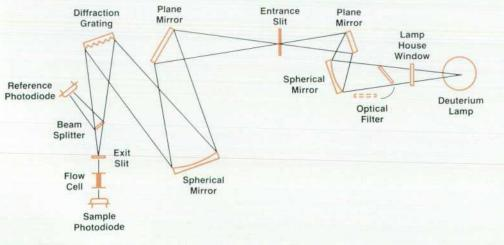
Fig. 2. Optical system of the HP 79853A Programmable Variable Wavelength Detector, a forward optics, scanning absorbance detector.
