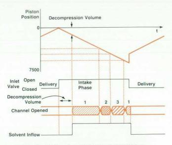
Fig. 13. Position dependent solvent proportioning
