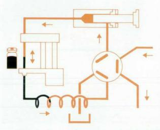
Fig. 5. Loading a partial sample into an extended seat capillary.
