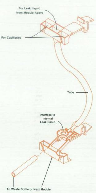
Fig. 1. Leak drainage system.
