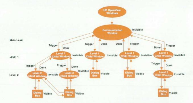
Fig. 3. Structure of the user interface module DTCMGRUI.
