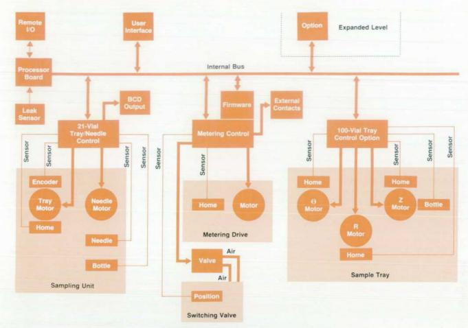
Fig. 8. Autosampler electronic block diagram.
