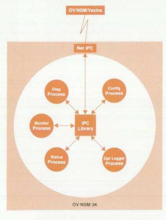
Fig. 2. The main components of the HP OpenView Network Services Monitor/3000 (OV/NSM/3K). The Diag process provides the diagnostic functions for troubleshooting a specific network problem. The Diag process is started by the Monitor process when a valid logon
