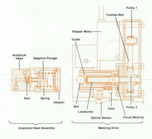
Fig. 7. Cutaway view of the metering device.
