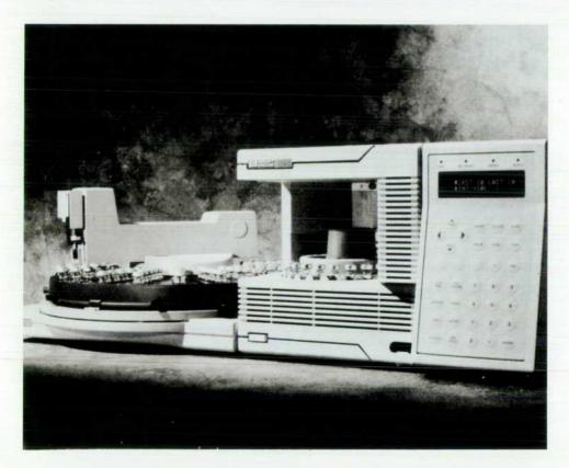
Fig. 9. Injector with 100-vial tray.
