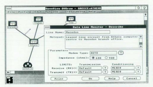
Fig. 4. The Describe dialog box is used to describe datacom line characteristics. The pencil is used to select the desired line.
