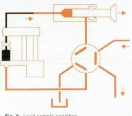
Fig. 3. Load-sample condition.
