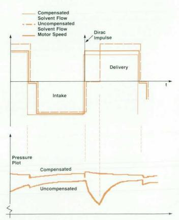
Fig. 8. Influence of ripple compensation on the pressure plot.
