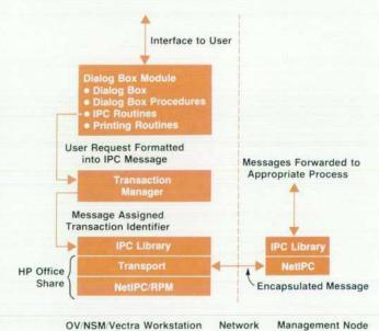
Fig. 5. The modules involved in providing interaction with the user and interaction with the network in the OV/NSM/ Vectra software. application's main window and posts all messages destined for an application to this queue, all messages resulting from user interaction with the map and menu items are received by HP OpenView Windows. HP OpenView Windows then forwards messages that arrive in its queue to the appropriate application's communication window for subsequent processing.
