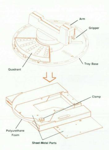
Fig. 10. HP 1050 Series support for the 100-vial tray.
