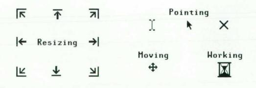
Fig. 1. Different pointer shapes that provide visual cues to the type of activity.
