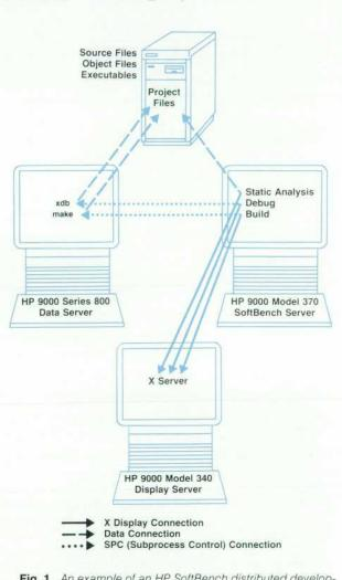
Fig. 1. An example of an HP SoftBench distributed development environment.
