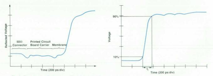
Fig. 8. Time-domain reflectometry profile and characteristic impedance.
