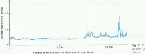
Fig. 7. Contact resistance as a function of the number of touchdowns.
