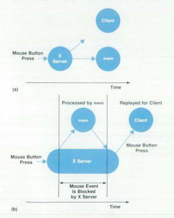
Fig. 10. (a) Mouse input stolen by mwm using a passive grab. The short arrow indicates that the button event never makes it to the client. (b) Mouse input intercepted by mwm and replayed. manager is running remotely.
