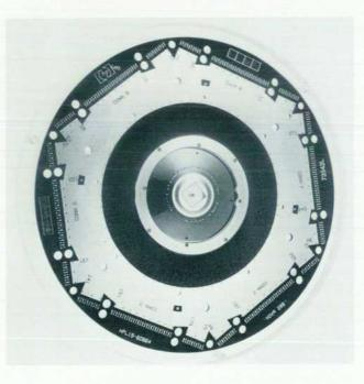
Fig. 16. The membrane probe for microprocessor testing.
