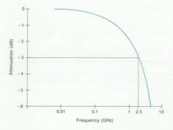
Fig. 10. Bode plot and the 3-dB bandwidth.
