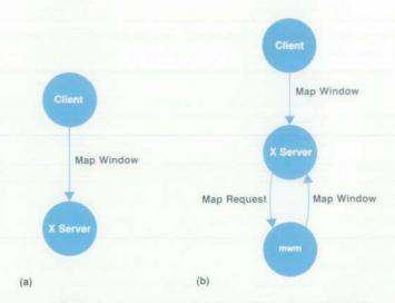
Fig. 4. Event redirection. (a) If no window manager is running (no redirection), the client's window mapping is done immediately. (b) When mwm is running, the server redirects the client's map window request to mwm. Mwm adds its window border before asking the server to complete the window mapping.
