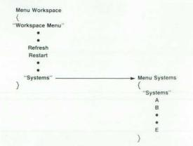
Fig. 11. The Systems menu is cascaded from the Workspace menu because of the entry in Workspace that calls the Systems menu.
