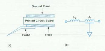
Fig. 1. Conventional wafer probe. (a) Structure. (b) Equivalent circuit. situations the same criterion is formulated differently; namely, one is faced with a high-speed testing situation when the DUT switches faster than the time constant of the circuit containing the parasitic reactance.
