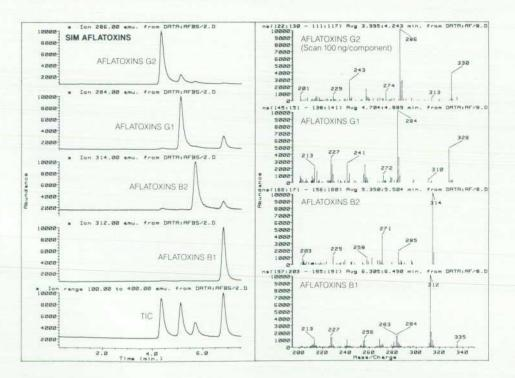
Fig. 13. Separation of aflatoxins by particle beam LC/MS.
