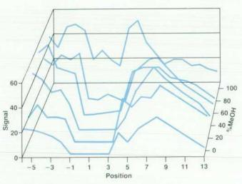
Fig. 4. Signal intensity for 10-ng injections of caffeine as a function of nebulizer position and mobile phase.
