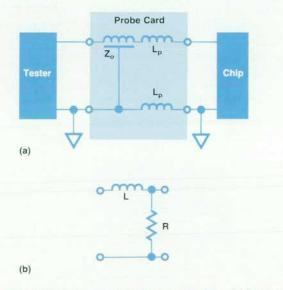
Fig. 2. The conventional probe as a signal line. (a) Equivalent circuit. (b) Equivalent low-pass filter.
