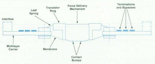
Fig. 6. Architecture of the membrane probe card. in Fig. 6. The membrane, configured as described above, is attached to a printed-circuit-board carrier, which also carries termination resistors, bypass capacitors, or any other necessary components. A force delivery mechanism is mounted on the printed circuit board carrier and is designed to perform three distinct and independent functions:
