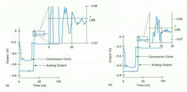
Fig. 15. Settling time of the DAC analog output. (a) Conventional probe card. (b) Membrane probe card
