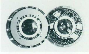
Fig. 14. The membrane probe for DAC testing.
