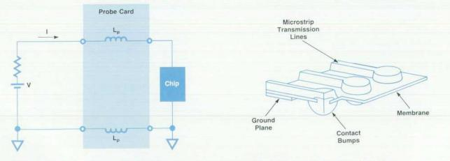
Fig. 4. A power line in a conventional probe.
