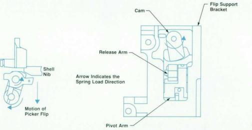
Fig. 9. Flip latch mechanism.
