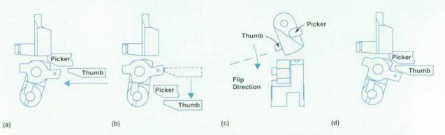
Fig. 10. Flip latch operation. (a) Initiation of flip. Thumb pushes release arm. (b) Start of flip. Picker falls through. (c) Start of cam opening. (d) End position of flip. Release arm cocked.
