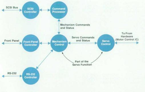
Fig. 2. Top-level firmware architecture. to control the motor voltage and receive positional feedback.
