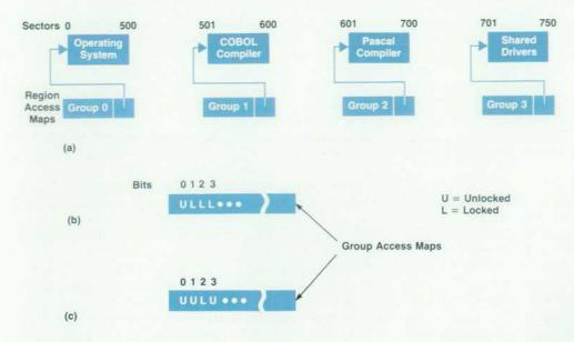
Fig. 3. (a) A typical group of files on a software distribution disk and their group associations. (b) Group access map showing that the customer has access to the operating system but not the COBOL or Pascal compilers. (c) Group access map showing that the customer has access to the operating system, the COBOL compiler, and the shared drivers.
