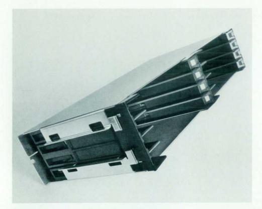
Fig. 12. One of the four eightcartridge magazines. Cantilever springs and snap details to hold the cartridges are molded into the plastic side parts of the magazines.
