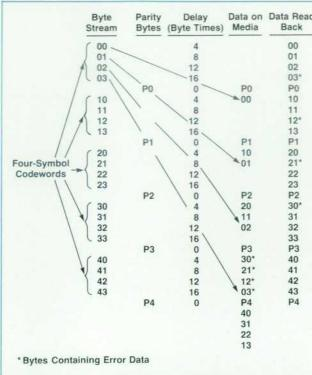
Fig. 4. Time-domain interleaving example.
