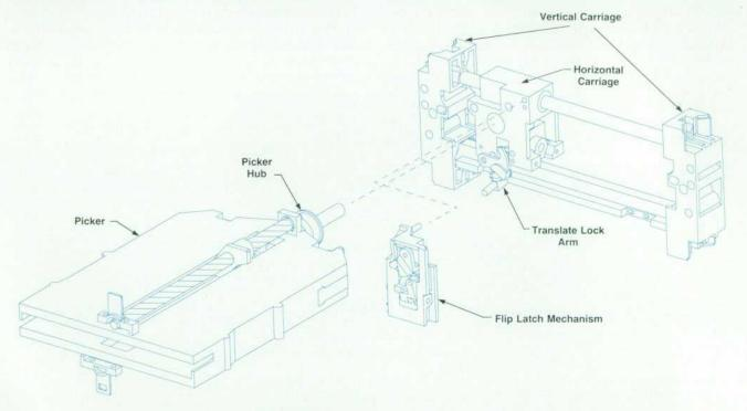
Fig. 7. Cartridge retrieval mechanism.
