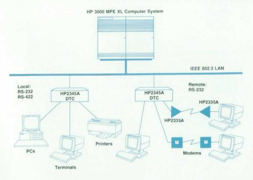
Fig. 1. The original HP 2345A distributed terminal controller could be thought of as a remote multiplexer. transport layer carries terminal I/O requests that are encoded using another proprietary protocol, ADCP, which manages all the terminal read, write, and control functions. It has also been optimized for performance.
