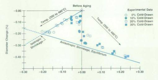
Fig. 4. Effect of aging temperature on the dimensional change of Cu 1.8 wt% Be. Aging time 2 hours.
