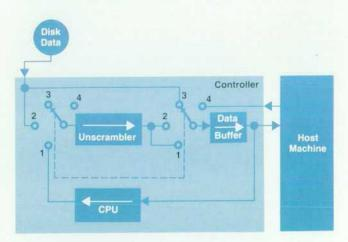
Fig. 4. Steering unscrambled data in and around the Model 600/A's unscrambler.
