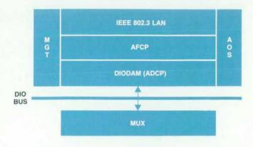
Fig. 2. Software architecture of the original DTC. AOS is the operating system. AFCP and ADCP are proprietary protocols.
