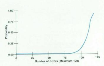
Fig. 7. A graph resulting from 21,150 passes through an unrecoverable data test algorithm. The graph shows the probability of unrecoverable data based on the number of errors.
