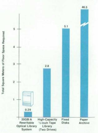
Fig. 4. Storage space comparison for 20.8 gigabytes.
