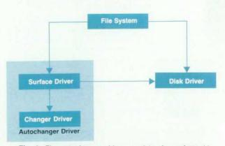
Fig. 1. The autochanger driver consists of a surface driver and a changer driver. The existing disk driver is used to control the optical drives.
