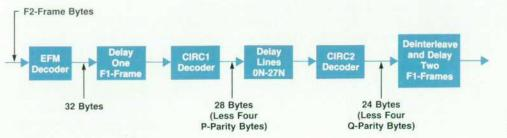
Fig. 4. CIRC error correction and decoding process.
