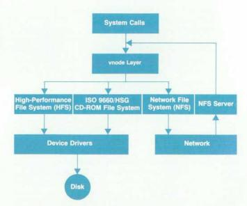
Fig. 5. The vnode architecture.
