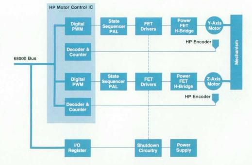
Fig. 1. Servo hardware architecture of the HP Series 6300 Model 20GB/A rewritable optical disk library system.
