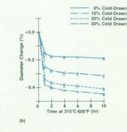
**Fig. 2.** Effect of aging time at 315°C on (a) axial and (b) transverse dimensional changes.
