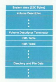
Fig. 1. The ISO 9660/HSG data layout on a CD-ROM disk.
