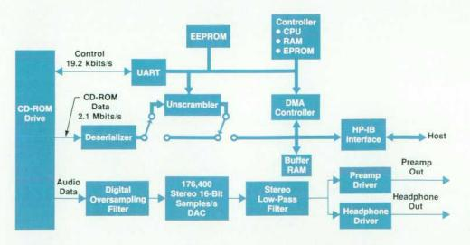
Fig. 6. The Model 600/A CD-ROM controller.
