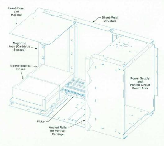
Fig. 1. Mechanical layout of the HP Series 6300 Model 20GB/A rewritable optical disk library system. subsystems.
