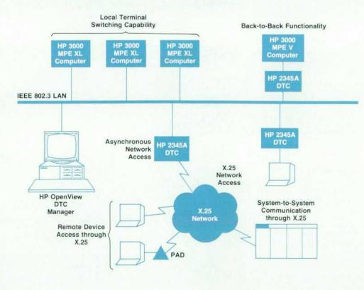
Fig. 3. The second-release HP 2345A DTC, renamed the data communications and terminal controller, offers X.25 network access, the ability of terminals to switch from one host to another, and back-to-back access to MPE V systems on the LAN. network management architecture. The management features include:
