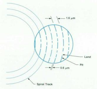
Fig. 1. A portion of a CD-ROM surface (not to scale).
