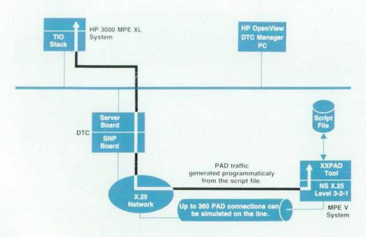
Fig. 9. The XXPAD tool was developed to test the PAD support software in the DTC without excessive hardware. The tool can simulate multiple connections. The first versions ran on an MPE V system.
