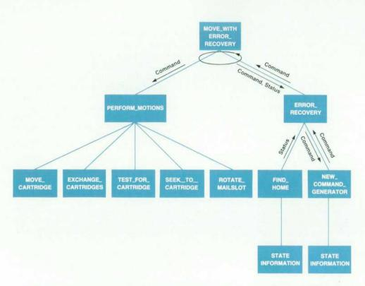
Fig. 4. Simplified hierarchical diagram of the motion control and error recovery firmware.
