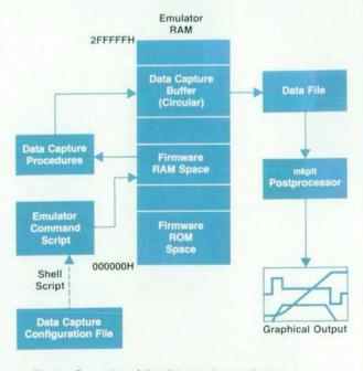
Fig. 1. Operation of the data capture system.
