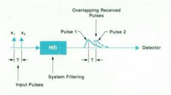
Fig. 7. Intersymbol interference. The incoming pulses overlap, making data detection more difficult. H(f) is the equivalent transfer function for all the filtering effects in the system (i.e., the transmitting filter, the channel filter, and the receiving filter).
