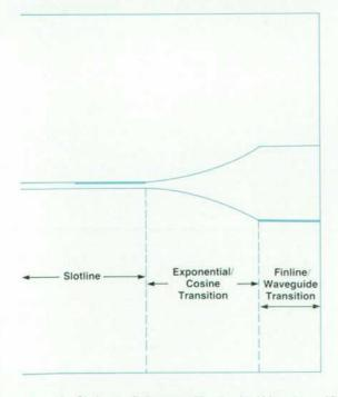
Fig. 13. Slotline-to-finline transition in the V-band amplifier doubler.
