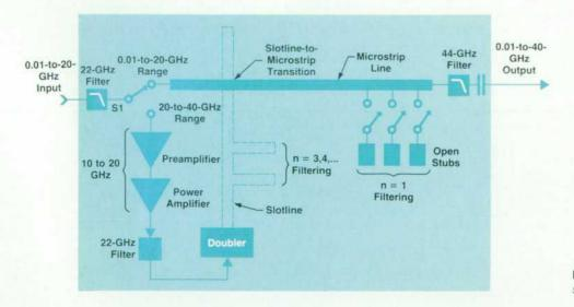
Fig. 1. Block diagram of the switched doubler microcircuit.
