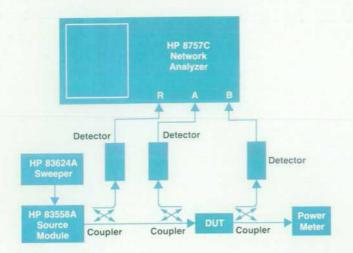
Fig. 23. Typical scalar network analyzer system.
