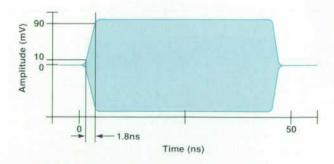
Fig. 6. Typical pulse envelope.
