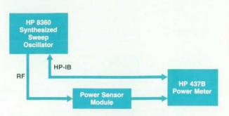
Fig. 1. The direct control method of power calibration.
