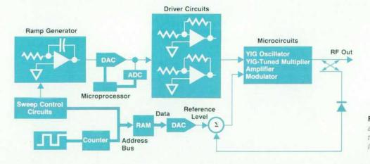
Fig. 4. The HP 8360 ramp generator adds digital control circuitry to provide 1601 ALC reference levels during a sweep.
