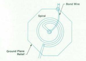
Fig. 8. Details of the spiral inductor used in the quasi-elliptic low-pass filters.
