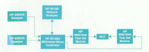
Fig. 25. HP W85106B vector network analyzer system.
