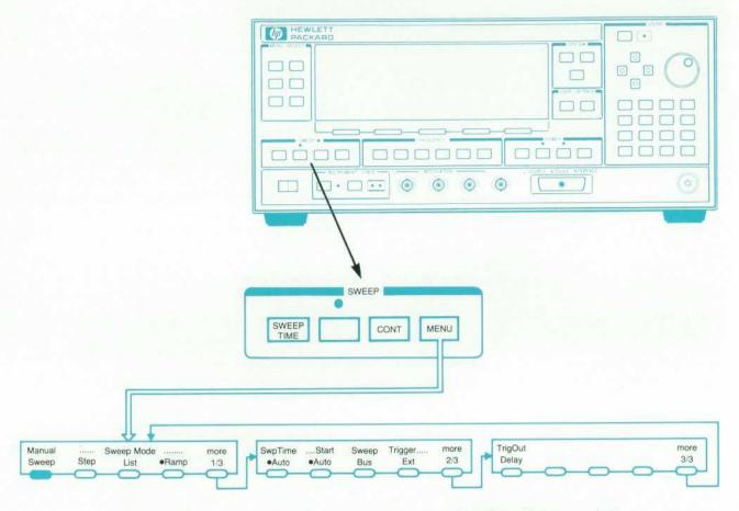
Fig. 6. HP 8360 menu concept. Similar functions are grouped together, with a menu select key as part of each group. The concept provides clear single-key access to the most often used features and places the less often used functions on the associated menu.
