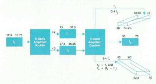
Fig. 19. Harmonic analysis for the V-band source module.
