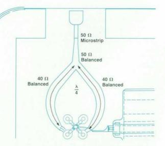
Fig. 7. Details of the LO balun in the triple-balanced mixer.
