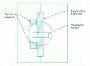
Fig. 14. Split block design of the finline-to-waveguide transition of the V-band amplifier doubler.
