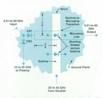
Fig. 3. Slotline-to-microstrip transition. Including the RF switch (CR1 and CR2) minimizes loss.
