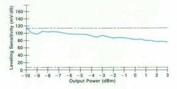
Fig. 18. Leveling sensitivity of the V-band source module.
