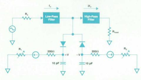
Fig. 10. W-band tripler with bias circuit.
