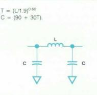
Fig. 2. Inductor model used in filter design.
