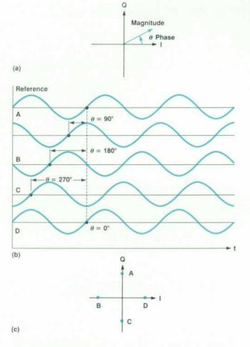
Fig. 2. (a) The I-Q plane. (b) Signals of varying phase. (c) Their I-Q diagram. This type of I-Q diagram is also called a constellation diagram.
