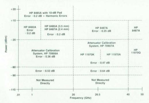
Fig. 6. A map of the equipment used for factory calibration of the HP 8360 output power and the measurement uncertainty.
