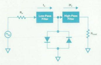
Fig. 7. Diode tripler antiparallel configuration.
