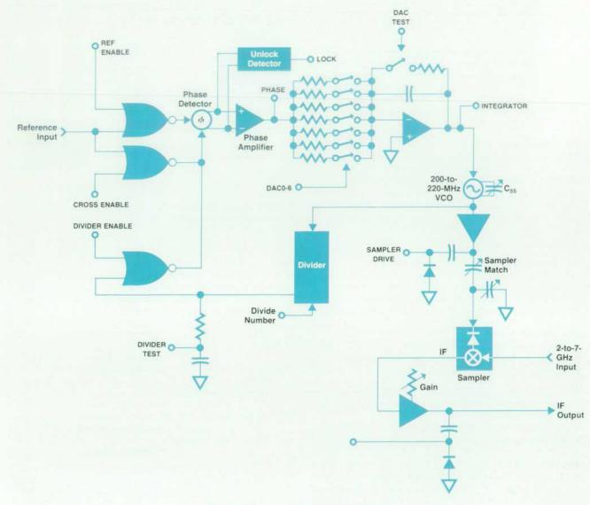
Fig. 2. Sampler driver phase-locked loop
