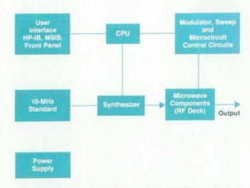
Fig. 2. Basic block diagram of an HP 8360 synthesized sweeper.
