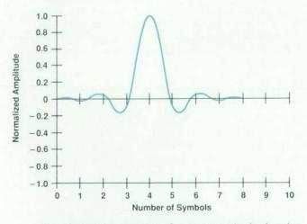
Fig. 10. Impulse response of a square root raised cosine filter with an  $\alpha$  of 0.35.
