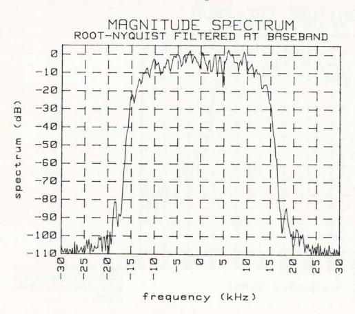
Fig. 6. A typical HP 11847A plot of the spectrum of a signal that has been down-converted and passed through a square root raised cosine filter.
