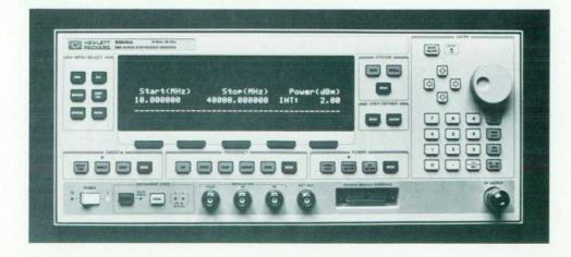
Fig. 1. HP 8360 synthesized sweep oscillators include eleven models that cover the frequency range from 10 MHz to 50 GHz. Millimeter heads extend the frequency range to 110 GHz (Model 83640A shown). High-powermodels provide 17 dBm at 20 GHz. Analyzer models have special network analyzer synchronization features. frequency control circuits, which correct the sweep inaccuracies. This automatic calibration feature has resulted in a tenfold improvement in swept frequency accuracy.
