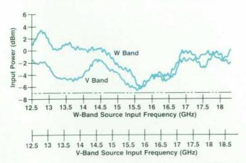
Fig. 17. Input power for – 2-dBm output power for the V-band source module and for – 5-dBm output power for the W-band source module.
