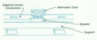
Fig. 2. Attenuation section with ground planes removed.
