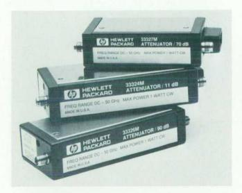
Fig. 1. The programmable coaxial attenuators used in the HP 8360 synthesized sweepers are also available as the HP 33324/26/27 programmable step attenuators. They operate from dc to as high as 50 GHz and provide up to 90 dB of attenuation in steps of 1 dB or 10 dB.
