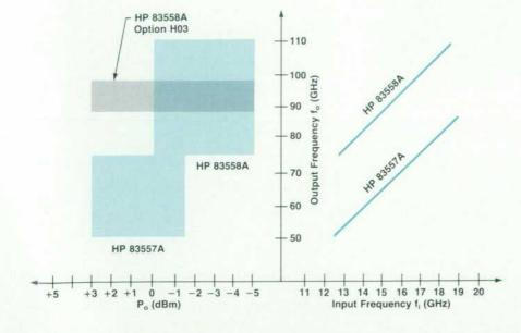
Fig. 3. Output power and frequency ranges of the new millimeter-wave source modules.
