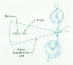
Fig. 9. Radial transmission line resonator used in the quasi-elliptic low-pass filters.
