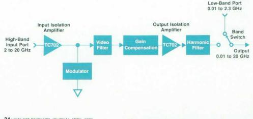
Fig. 1. Block diagram of the fast pulse modulator.
