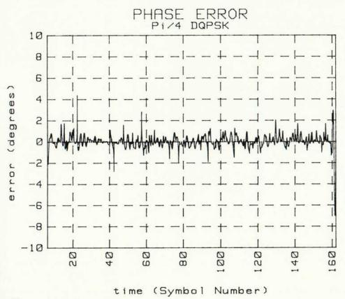
Fig. 9. HP 11847A plots (a) magnitude error and (b) phase error. (Fig. 9 continued on next page.)
