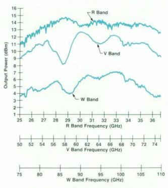
Fig. 16. Typical output power of the W-band amplifier tripler, the V-band amplifier doubler, and the R-band amplifier doubler.
