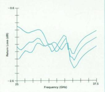
Fig. 2. Diode return loss predicted by the HP Microwave Design System at three power levels.
