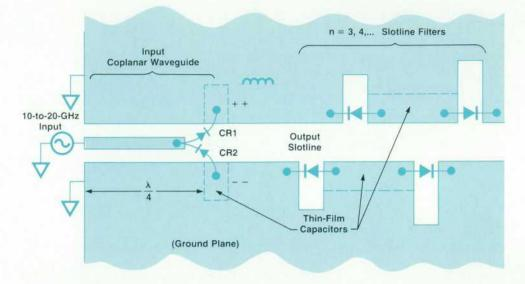
Fig. 2. Doubler and slotline filter structure.
