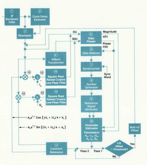
Fig. 3. The HP 11847A signal processing flow diagram.
