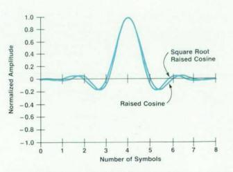
Fig. 11. Comparison of raised cosine and square root raised cosine filter with  $\alpha = 0.35$ .
