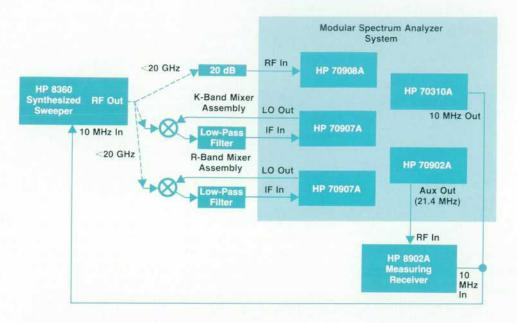
Fig. 7. Attenuator calibration system for calibrating the HP 8360 output power at low power levels.
