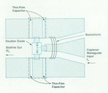
Fig. 12. Coplanar waveguide input structure.
