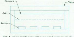
Fig. 1. Basic construction of the vacuum fluorescent display used in the HP 8360 synthesized sweepers. Shock testing was done in six axes with an initial level of 30g for a duration of 11 milliseconds.
