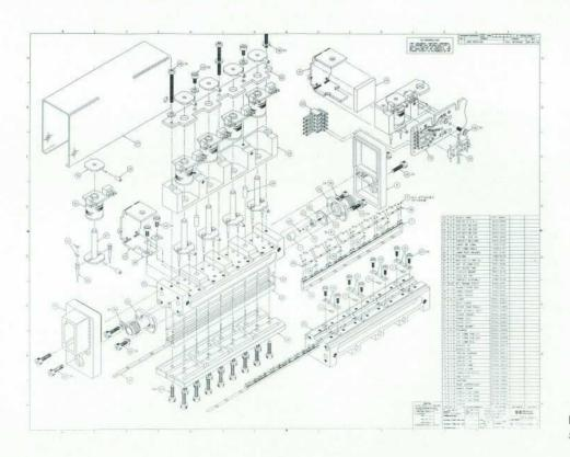
Fig. 4. Exploded view of a foursection attenuator.
