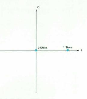
Fig. 3. On/off keying I-Q diagram.
