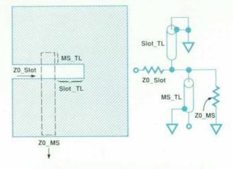
Fig. 15. Slotline-to-microstrip transition of the R-band amplifier doubler with circuit model.
