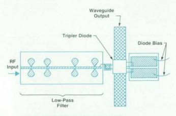
Fig. 8. Physical layout of the diode tripler.
