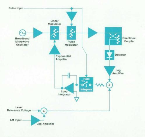
Fig. 1. The type of ALC loop used in the HP 8340 synthesized sweep oscillator. cuted whenever the frequency or the power level is changed, so the response is slow. Without feedback, the power level drifts with time and the AM accuracy is poor.
