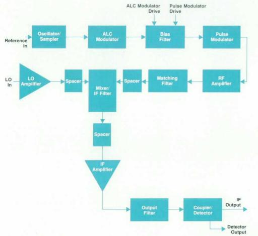
Fig. 4. Functional block diagram of the low-band microcircuit.
