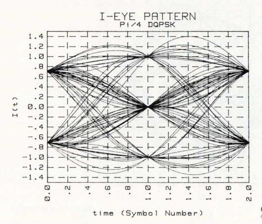
Fig. 8. A typical I-channel eye diagram.
