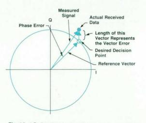
Fig. 14. I-Q diagram showing the parameters used to compute the vector error.
