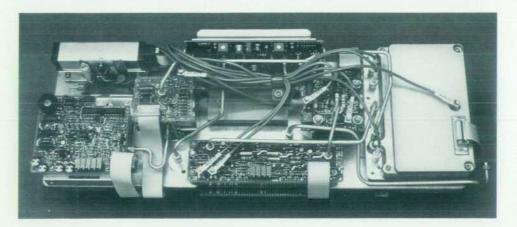
Fig. 4. The RF deck holds all of the microwave components. For rear-panel input/output options, the deck is reversed to keep microwave path lengths as short as possible.
