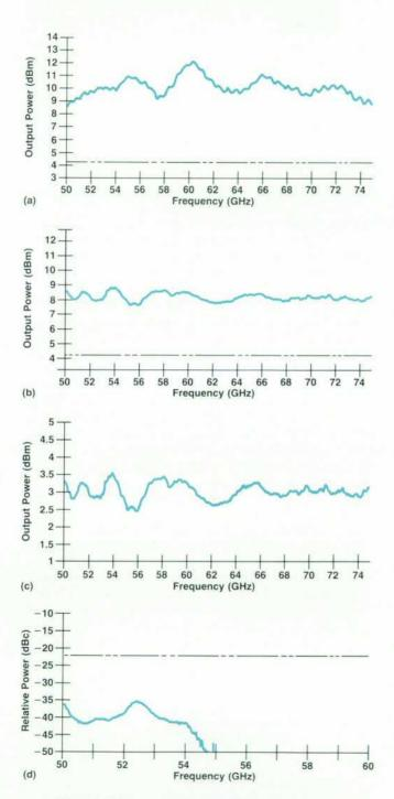
Fig. 21. Typical performance of the HP 83557A V-band source module. (a) Typical unleveled output power. (b) Typical leveled output power. (c) Typical flatness at +3-dBm output power. (d) Typical harmonic performance (5/4 harmonic).
