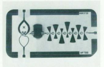
Fig. 10. Fifteen-pole quasi-elliptic low-pass filter.
