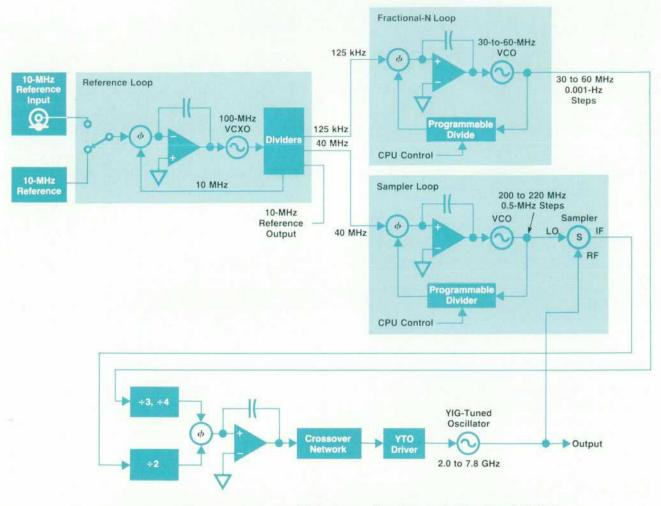
Fig. 3. HP 8360 frequency synthesizer block diagram. The phase-locked loops are locked at the beginning of a sweep so the start frequency has synthesizer accuracy. The loops are unlocked for continuous sweeping. An end-of-sweep calibration with synthesizer accuracy provides a tenfold improvement in overall swept frequency accuracy over previous designs.
