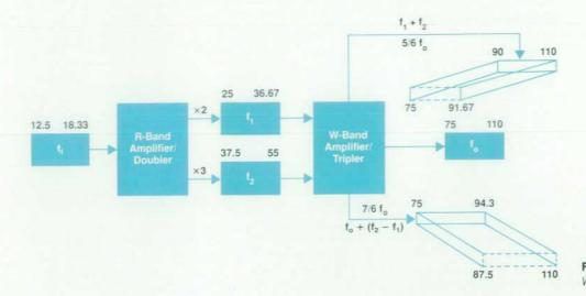
Fig. 20. Harmonic analysis for the W-band source module.
