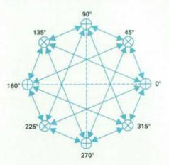
**Fig. 6.** Unfiltered phase transitions for  $\pi/4$  DQPSK. The trajectories inside the octagon represent 135° transitions. For example, from 0° there can be a transition to 135° or 225°. The arrows around the outside of the octagon represent 45° transitions.
