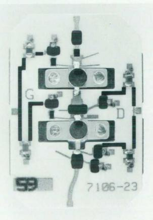
Fig. 2. The LO amplifier of the low-band microcircuit is an example of a circuit with no bonds. Connections are made by integral contacts on the package lid.
