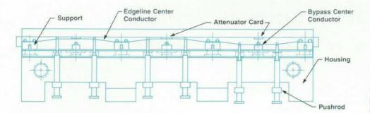
Fig. 3. Cutaway side view of a three-section attenuator with solenoids removed.
