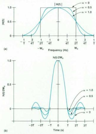
Fig. 8. Raised cosine filter characteristics. (a) System transfer function for several values of  $\alpha$ . The  $\alpha = 0$  roll-off is the minimum bandwidth case. (b) System impulse response.
