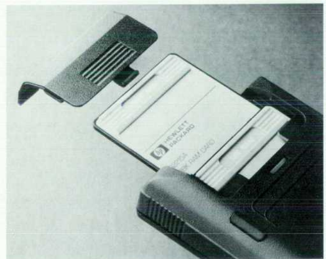
Fig. 1. Two expansion ports accept ROM or battery-backed RAM cards.
