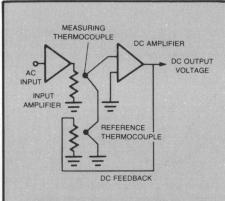
Figure 5. A thermal true rms converter uses dual matched thermocouples operated in opposition to cancel the effects of ambient temperature and to produce a linear output.
