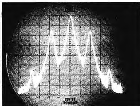
Figure 4. LOG Display of Amplitude Modulated Carrier. SCAN WIDTH is 200 Hz/div; IF BANDWIDTH is 50 Hz. The modulation frequency is measured directly from the display as 400 Hz (2 division spacing of carrier and sidebands). The modulation percentage is measured from the 16 dB amplitude ratio of the carrier and sidebands . . . modulation percentage is 30%. The 800-Hz second harmonic distortion components are 40 dB below the fundamental, indicating 1% distortion. The calibrated LOG display also shows the carrier level to be -31 \text{ dBm} (see Figure 5).
