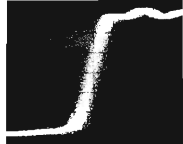
Fast rise time pulses are used as standards to check the rise time of oscilloscopes, amplifiers, and components. Fast step is also used in Time Domain Reflectometry.
