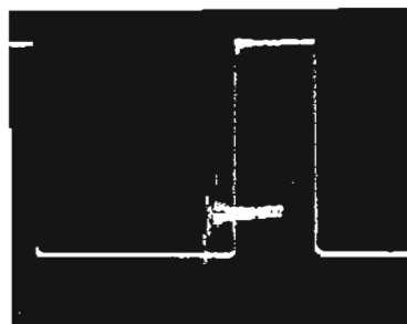
Double exposure showing 5-cm pulse on upper waveform, and the same pulse expanded 10 X to view small perturbation on the top.
