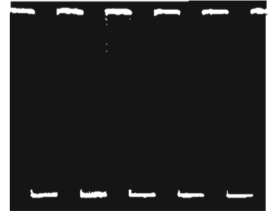
The square wave is useful in amplifier testing and calibration, and attenuator checking.
