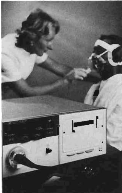
Ear Oximeter measures O 2 saturation non-invasively, continuously — independent of skin pigmentation, ear thickness, ear-plate motion. No individual patient calibration needed.
