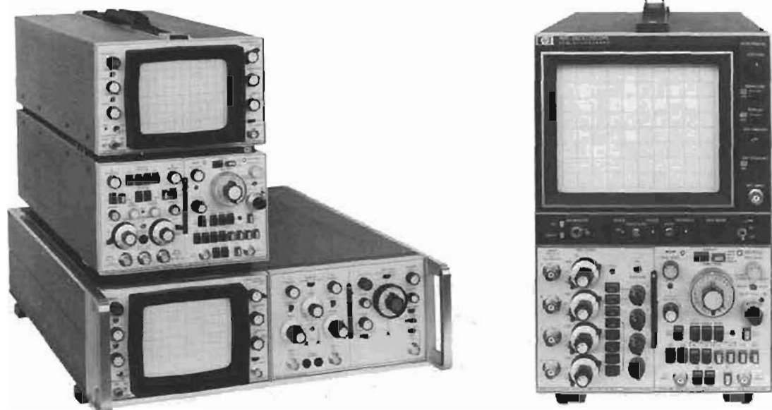
Figure 1. Representative plug-in oscilloscopes from Hewlett-Packard's 180 series.
