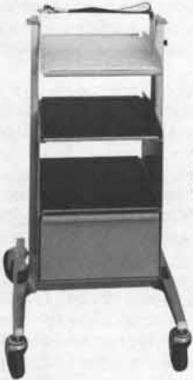
Opt 006: storage cabinet with shelf on top, and drawer in lower position, load limit 18 kg (40 lb) on shelf, 18 kg (40 lb) in cabinet, and 11 kg (25 lb) in drawer.
