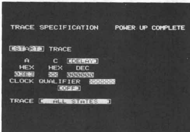
Figure 5. Trace Specification menu (resulting from the Format Specification in figure 4) shows the labels assigned and the numerical base in which to enter data. This Trace Specification defines that the trace point will start data collection when address 03E3 16 is recognized.
