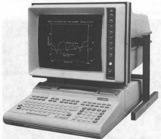
1311A Option 010 demonstrates the high tilt stand which allows a 9825A desktop computer or 1350A graphics translator to be positioned beneath the 1311A display.
