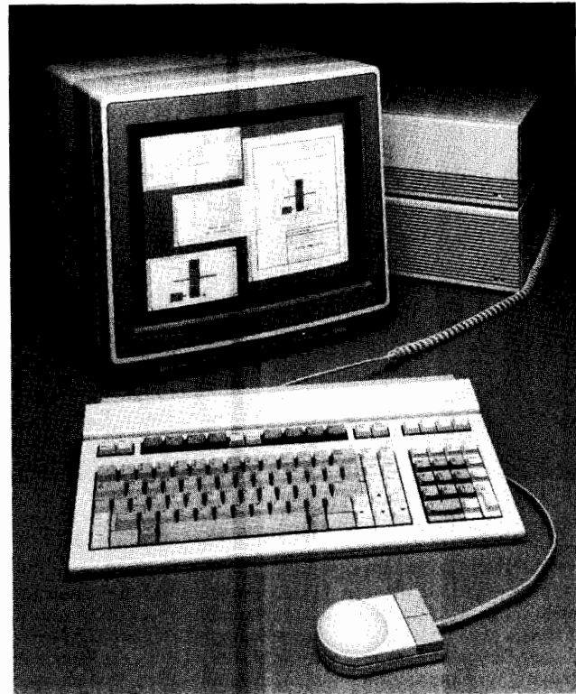
The HP 85150A Microwave Design System runs on a compact workstation to design microwave components quickly and accurately.
