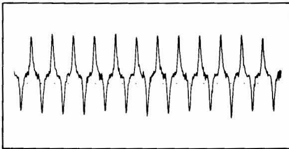
This signal was recorded from a floppy disc read head.
