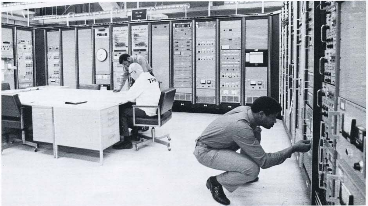
Banks of modern instrumentation provide a wide range of cell/battery test parameters. Here, test engineers are evaluating a computer analysis while parameters are being adjusted for another battery test.
