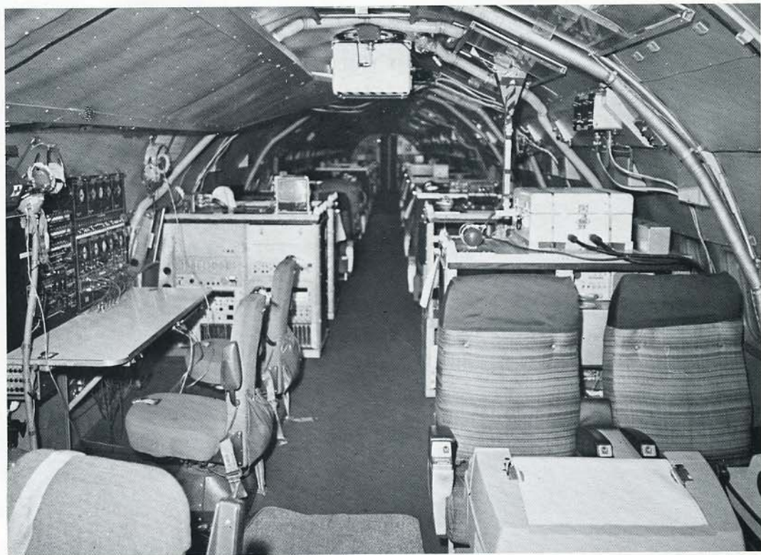
Scientific measuring instruments occupy most of the space onboard the research aircraft. At the left are the meteorological flight director's desk and control panel, and in the right foreground are the scientific control center's printer and typewriter.
