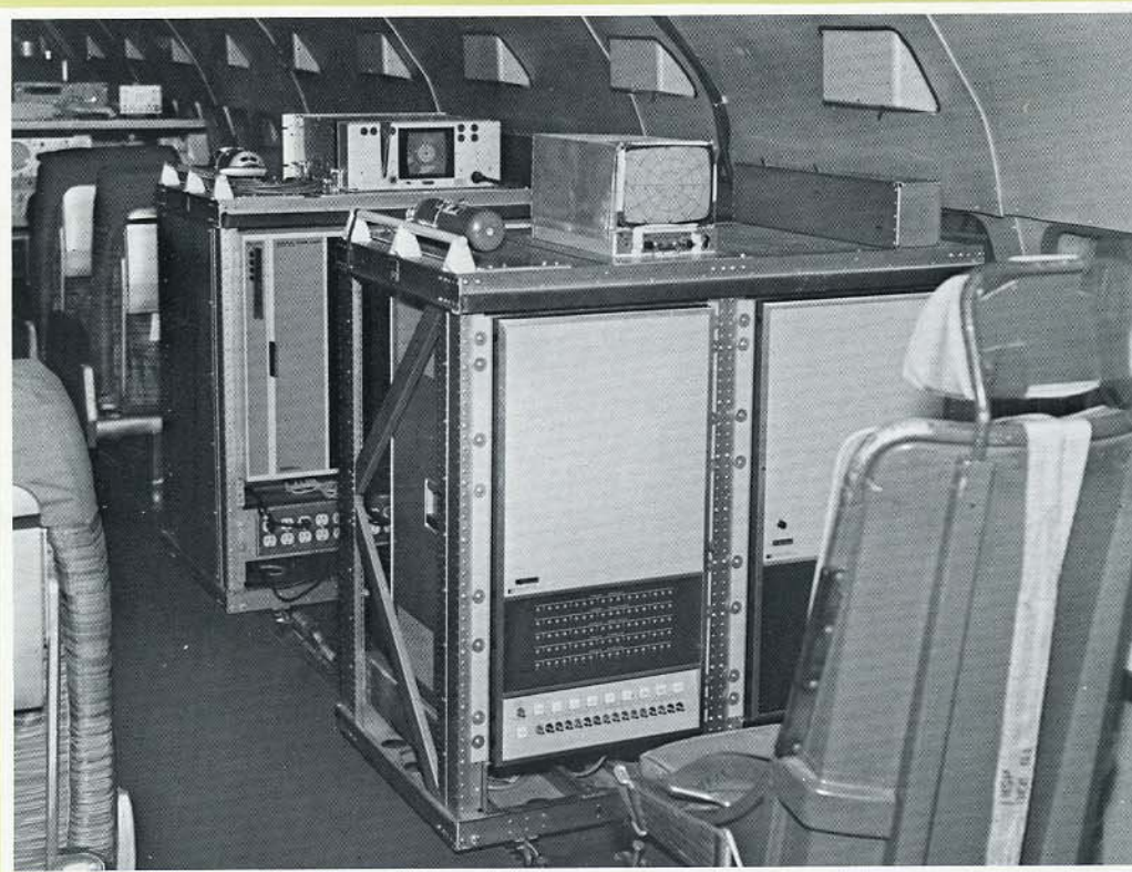
Onboard the NASA Research aircraft, an HP computer performs on-line data reduction and other functions to aid scientific observers in their data gathering missions.
