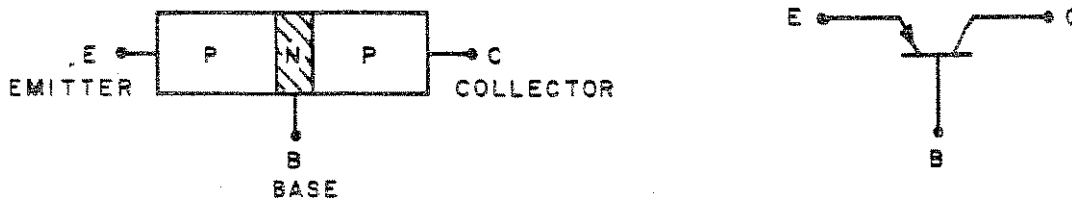
Figure 4-1. PNP Transistor and Circuit Symbol
