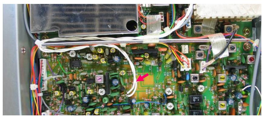
Solder a twisted pair of wires to the small resistor lead loops. Route neatly to back of radio.
