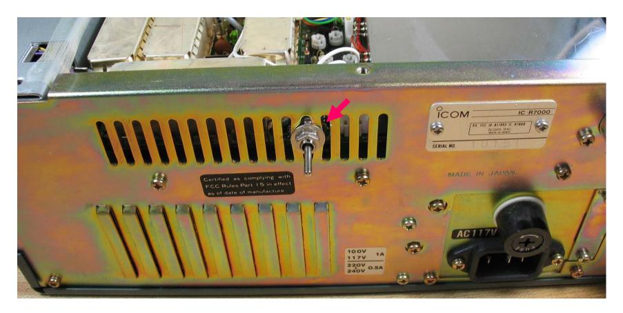
Terminate the two wires with a subminiature SPST toggle switch. Place switch through ventilation holes on back of IC R-7000
