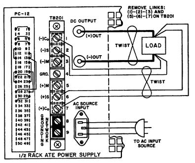
FIG. 3-5 LOAD CONNECTION, METHOD III.
