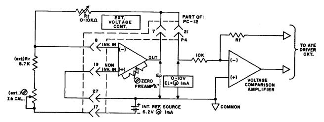
FIG. 3-7 TWO-TERMINAL RESISTANCE PROGRAMMING OF THE VOLTAGE CHANNEL, USING PREAMP "A" AND THE INTERNAL REFERENCE SOURCE.
