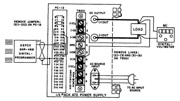
FIG. 3-6 OUTPUT VOLTAGE CONTROL WITH AN EXTERNAL (0-10V, 1 mA) D-C CONTROL SIGNAL.
