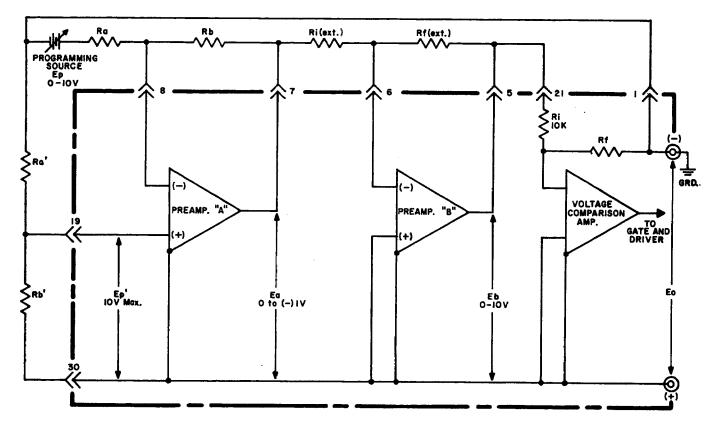
FIG. 3-29 PROGRAMMING WITH REFERENCE TO THE NEGATIVE OUTPUT SIDE OF THE ATE.
