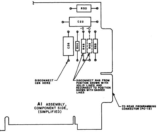
FIG. 3-27 LOCATION OF OVERVOLTAGE SENSING LEAD DISCONNECT.
