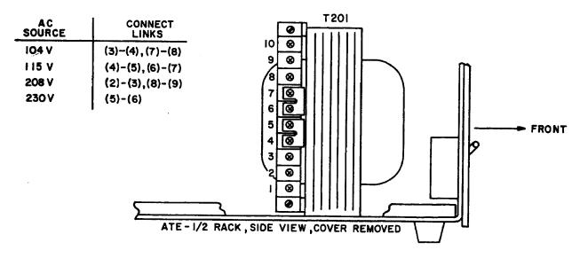
FIG. 24 A-C INPUT SOURCE VOLTAGE SELECTION, ATE 1/2 RACK GROUP.
