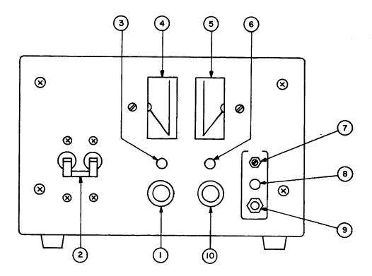
FIG. 2-2 CONTROL AND TERMINATIONS, ATE 1/2 RACK GROUP, FRONT.
