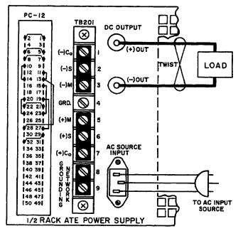
FIG. 3-3 LOAD CONNECTION METHOD I, LOCAL ERROR SENSING.
