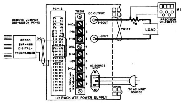
FIG. 3-11 CONNECTIONS FOR OUTPUT CURRENT CONTROL WITH A 0-1 VOLT CONTROL SIGNAL (KEPCO SN-488 DIGITAL PROGRAMMER).
