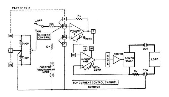
FIG. 3-1B BOP CURRENT CONTROL CHANNEL
