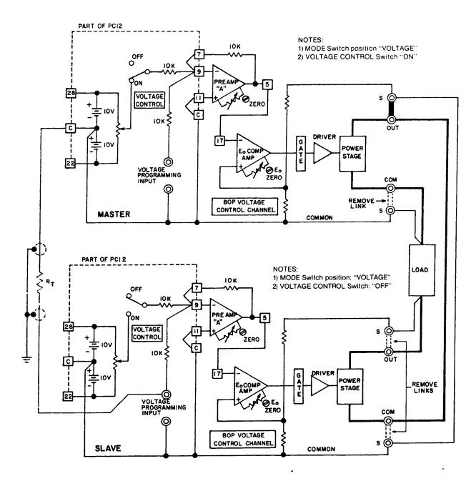
FIG. 3-26 MASTER/SLAVE SERIES CONNECTION OF TWO BOP POWER SUPPLIES, WITH ERROR SENSING AT THE COMMON LOAD.
