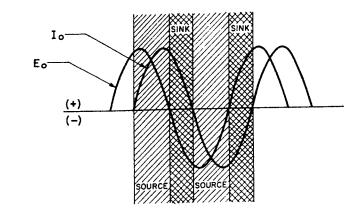
FIG. 1-3 BOP OUTPUT WAVE FORM WITH PHASE SHIFT
