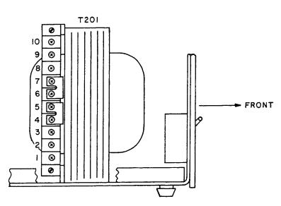
FIG. 2-3 A-C SOURCE VOLTAGE SELECTION.
