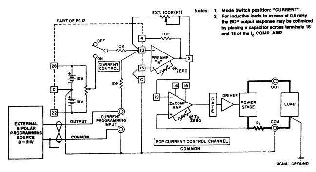
FIG. 3-18 PROGRAMMING CIRCUIT FOR DRIVING THE BOP OUTPUT CURRENT WITH A BIPOLAR SIGNAL LESS THAN ± 10V (EXAMPLE SHOWN: ± 1V SOURCE)
