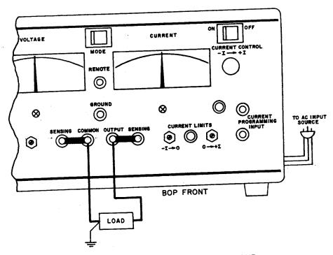
FIG. 3-2B LOAD CONNECTION AT THE FRONT, WITHOUT ERROR SENSING.
