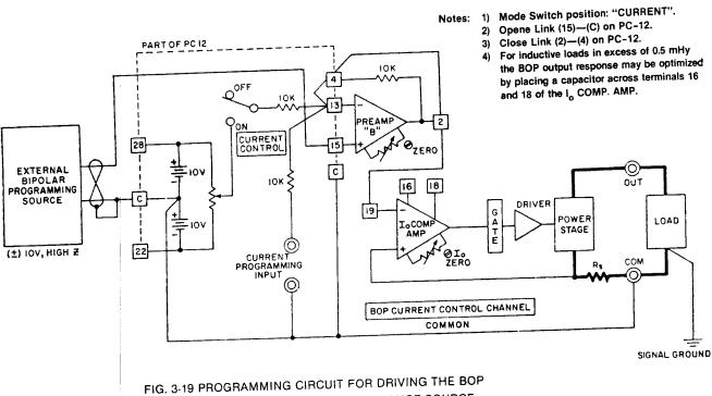
FIG. 3-19 PROGRAMMING CIRCUIT FOR DRIVING THE BOP OUTPUT CURRENT WITH A HIGH IMPEDANCE SOURCE
