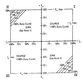
FIG. 1-2 BOP OUTPUT CHARACTERISTIC
