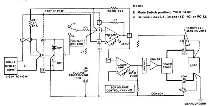
3-20 If, for example, the BOP d-c output is to be controlled by means of a bipolar, 1 volt, high impedance source, it can be connected to the BOP as shown in FIG. 3-7.
