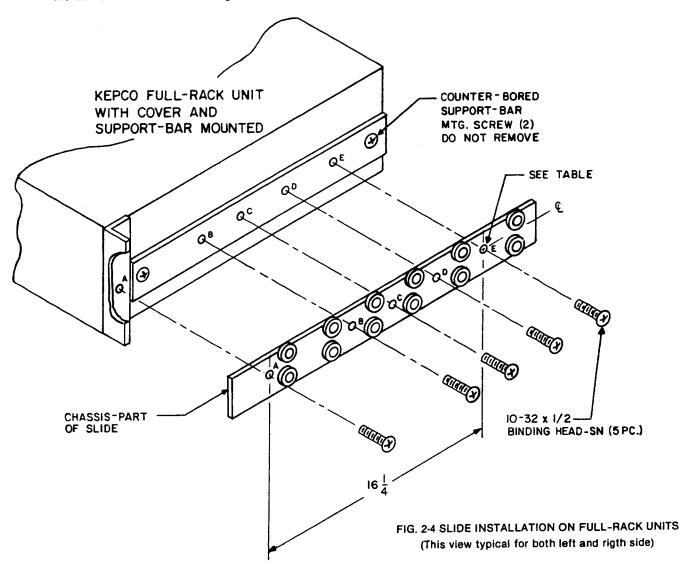
**NOTE:** If slide installation (as described above) is not desired, other means of supporting the unit in the rear must be provided (additional rear brackets or a solid platform, for example) since the front angle brackets alone are not sufficient to support the full weight of the unit.
