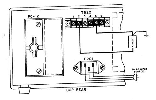
FIG. 3-2A LOAD CONNECTION AT THE REAR, WITHOUT ERROF: SENSING.
