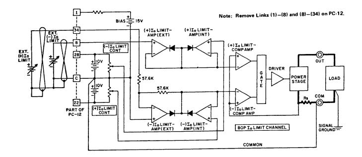
FIG. 3-22 INDEPENDENT REMOTE CONTROL OF THE BOP (+)  $I_0$  AND (-)  $I_0$  LIMITS
