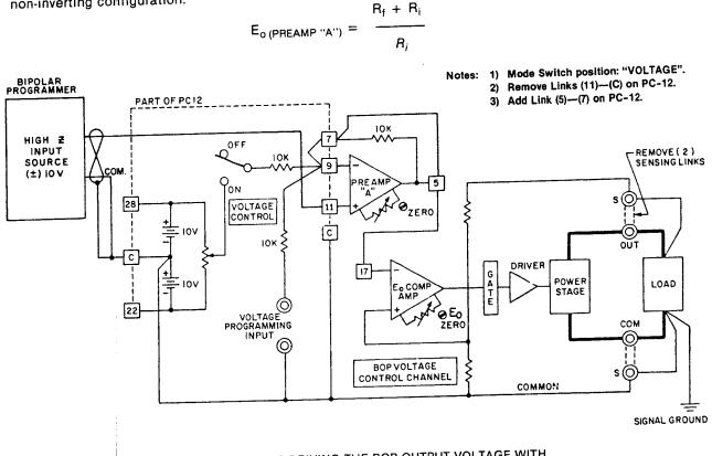
FIG. 3-11 PROGRAMMING CIRCUIT FOR DRIVING THE BOP OUTPUT VOLTAGE WITH A HIGH-IMPEDANCE SOURCE, USING THE NON-INVERTING INPUT OF PREAMP "A".
