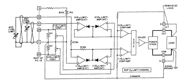
FIG. 3-25 INDEPENDENT REMOTE CONTROL OF THE BOP (+)  $E_0$  AND (-)  $E_0$  VOLTAGE LIMIT CIRCUITS
