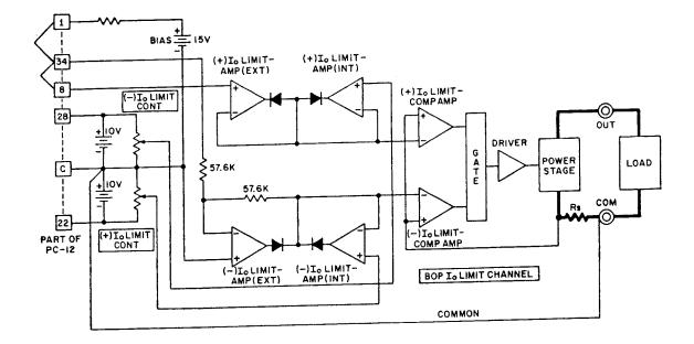
FIG. 3-1D BOP (±) CURRENT LIMITING CIRCUIT
