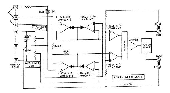
FIG. 3-1C BOP (±) VOLTAGE LIMITING CIRCUIT
