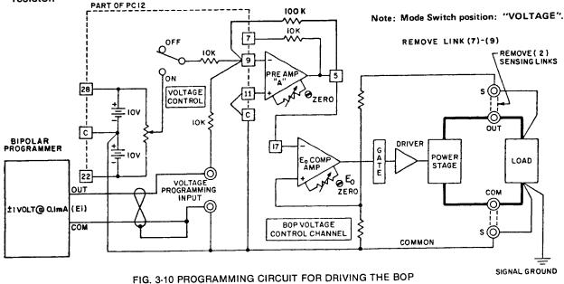
OUTPUT VOLTAGE WITH A BIPOLAR (± 1V) SIGNAL
