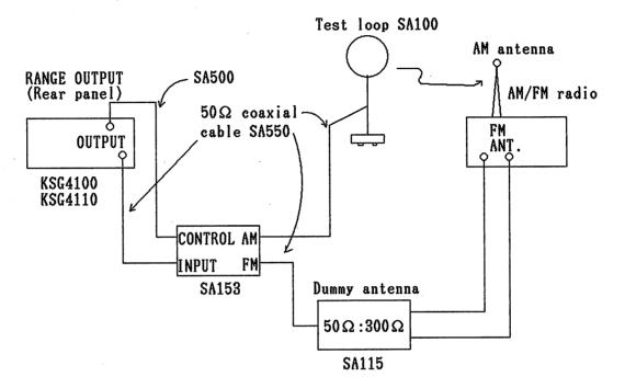
Figure 8-10 SA153 connection diagram
