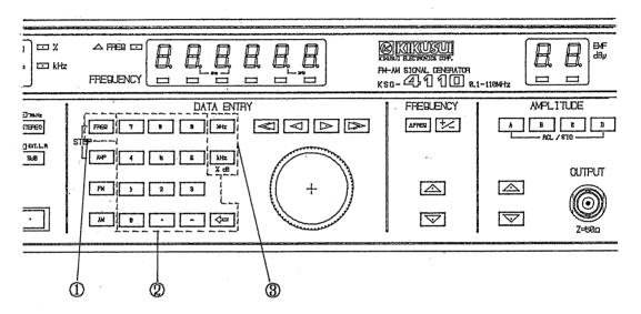
Press the **WRED** key and input the desired values using the Numeric Keys. Operate in the sequence indicated by the numerals (1), (2) and (3) in the diagram above.
