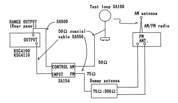
Figure 8-11 SA154 connection diagram
