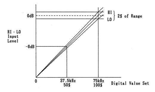
For example, if the input level is attenuated to -6dB after the input level is set in the **HI**, **HI** range and the display is set to 75kHz deviation, the display will be 75kHz = 100% and deviation becomes 37.5kHz = 50%. At this time, the **HI** lamp will light but normal 37.5kHz deviation will be obtained.
