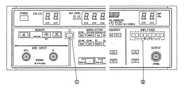
The four keys ② ③ to ③ shown in the diagram above can store output levels without using the main memory.
