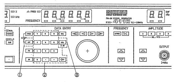
Press the key and continuously input desired values using the numeric keys. Operation is in the sequence ①, ②, ③ shown in the diagram above. If a key other than those shown inside the dotted lines is pressed, the value displayed before the key was pressed will again be displayed.
