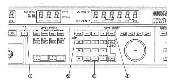
Input is set in the sequence (1), (2), (3), (4) shown in the diagram above.
