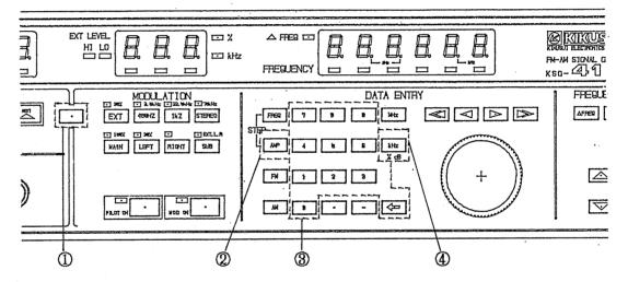
Input is set in the sequence (1), (2), (3), (4) shown in the diagram above.
