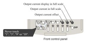
Fig.6-6 Current system adjustment variable resistor
