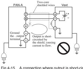
Fig.4-15 A connection where output is short-circuited by the shield
