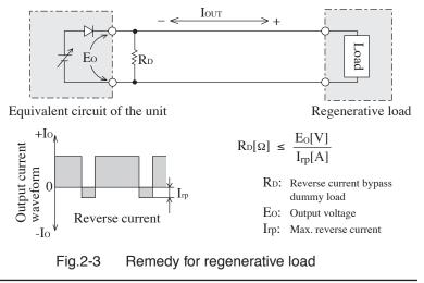
▲ CAUTION • For the resistor RD, select a resistor of the rated power (allowing sufficient margin). If a resister of insufficient rated power is used in the circuit, it may burn out.
