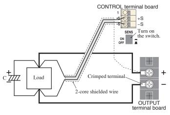
Fig.4-4 Remote sensing connection
