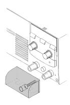
Fig.3-5 Mounting the auxiliary output terminal cover
