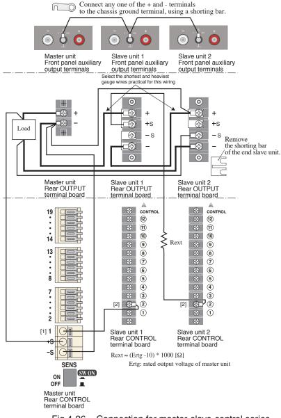
Fig.4-26 Connection for master-slave-control series operation using sensing (When the PAN-A and PAN series are used together)
