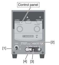
Fig.5-1 Front panel of PAN-A series model 175W
