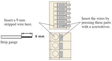
Fig.4-2 Connection to the control terminals
