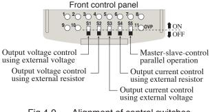
Fig.4-9 Alignment of control switches
