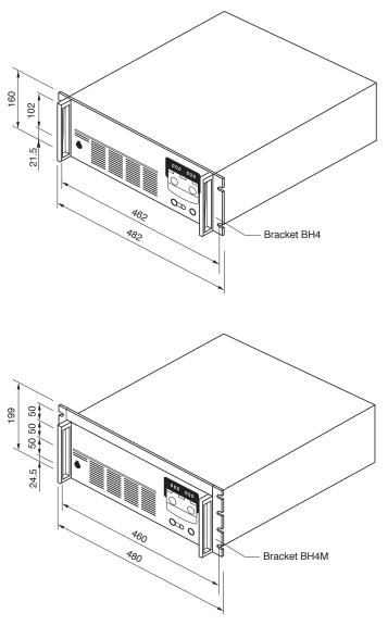
Fig.P-4 Model 1000W with BH4M/ BH4 mounted on it
