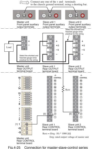
Fig.4-25 Connection for master-slave-control series operation (When the PAN-A and PAN series are used together)
