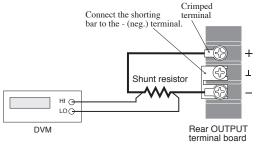
Fig.6-5 Connection for current system adjustment (PAN16-50A)
