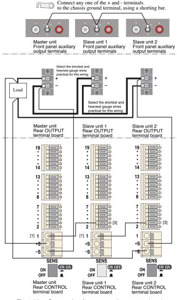
Fig.4-23 Connection for master-slave-control series operation using sensing
