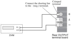
Fig.6-2 Connection for voltage system adjustment (PAN16-50A)
