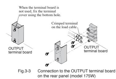
As shown in Fig.3-3, lay load cables at the left of the OUTPUT terminal board, as seen from the rear panel.
