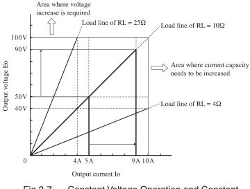
Fig.2-7 Constant Voltage Operation and Constant Current Operation
