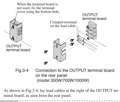
**NOTE** • The shape of the rear output terminal cover of the PAN16-50A is different from that shown in Fig.3-4.
