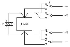
Fig.4-7 Power ON/OFF using mechanical switches
