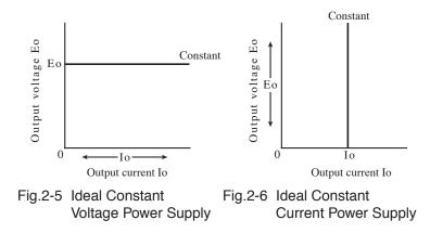
However, the output impedance of an actual constant voltage or constant current power supply is neither zero nor infinite, and they have a definite frequency response. In addition, maximum voltage or maximum current constraints on output are a factor, leaving these power supplies unable to maintain constant voltage or current with respect to all changes in load current or load resistance.
