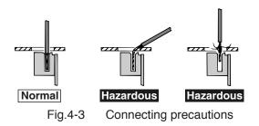
5. Remove the screwdriver from the terminal, and pull the wire gently to ensure that it is securely inserted.
