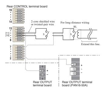
Fig.4-16 Output ON/OFF control connection
