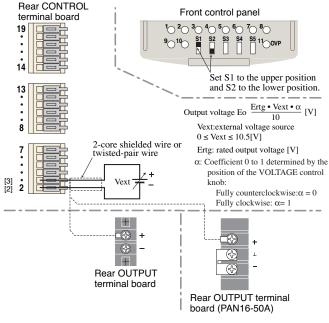
Fig.4-11 Connection and setup for output voltage control using external voltage
